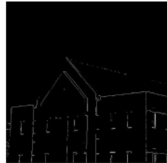
(d) Processed Image utilizing both vertical and horizontal Sobel mask with Specified Threshold
