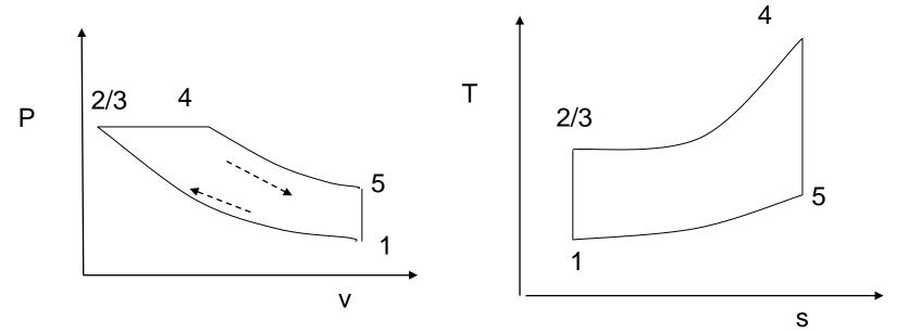
In Diesel cycle, there is only constant pressure heat addition. So points 2 and 3 are at the same location.
