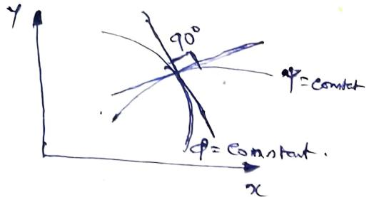
The orthogonality between streamlines helps to draw a flow net.
