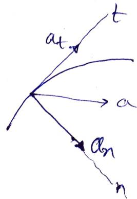
$$a_s = \frac{dv_s}{dt} = \frac{\partial v_s}{\partial t} + \frac{\partial v_s}{\partial s} \cdot \frac{ds}{dt} + \frac{\partial v_s}{\partial n} \cdot \frac{dn}{dt}$$
