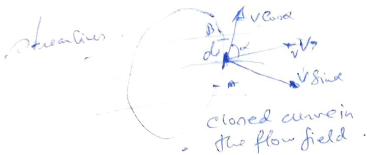
Circulation  $\Gamma$  is the line integral of tangential velocity around a closed contour in the flow field.
