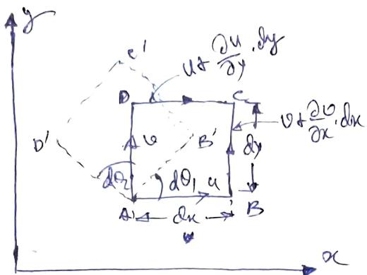
These different velocities will result into angular velocities of linear element AB,
