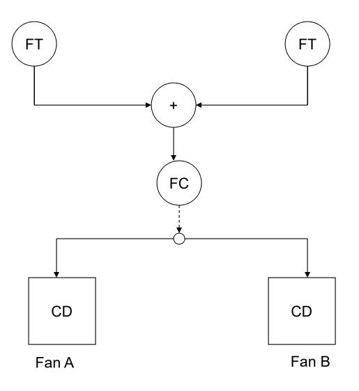
Control of air flow: Operation of FD Fans with single controllers
