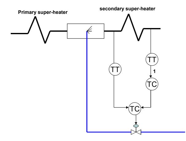
Steam temperature control: a typical cascade control action
