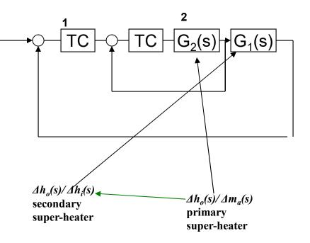
Time constants of each transfer function is  $\frac{\rho_{0_{ss}}V}{m_{o_{ss}}}$
