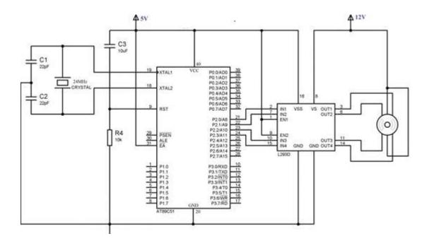
L293D is connected to pins P2.0, P2.1, P2.2, P2.3 of the microcontroller and two pairs of L293D are enabled by tieing EN1, EN2 to 5V. Logic Voltage (5V) is connected to Vss pin and Motor Supply (12V) is connected to the Vs pin of L293D. Each winding of the motor can be energized by making corresponding pin of L293D LOW.
