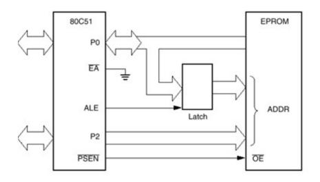
Program and Data memory are separate Program Memory can be internal and/or external.
