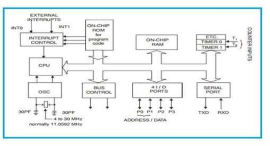
In the timer mode, the internal machine cycles are counted. This register is incremented in each machine cycle i.e. 12 clock cycles. For example, if the clock frequency is 12MHz, then the timer register is incremented in each millisecond. In this mode it ignores the external timer input pin
