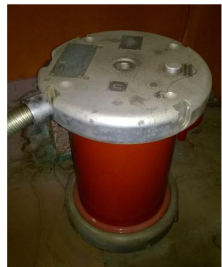
Figure 2.10 High Voltage Testing Transformer
