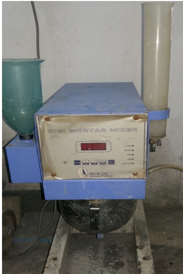
Figure-3.1 : Preparation of GGBFS Paste in Mortar Mixer
