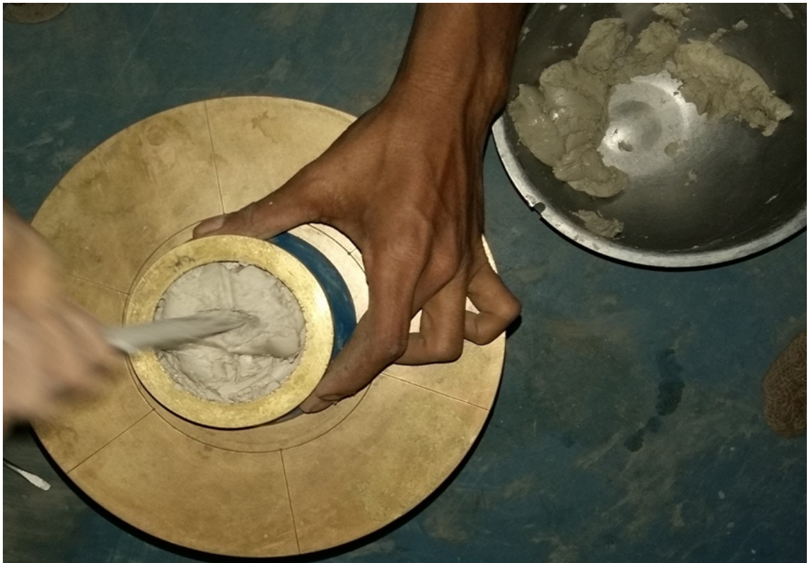
Figure 3.2: Mini flow table as per ASTM C1437-07
