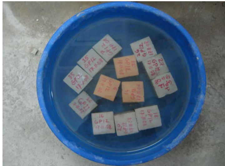
Figure-3.5: Setup for Water absorption test
