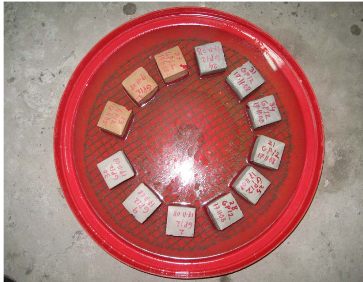
Figure-3.6: Setup for Water Sorptivity test
