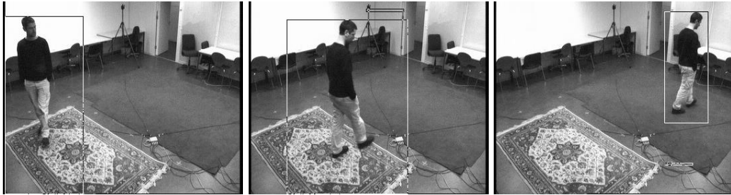
Fig. 21: Result of object tracking of 35 th , 100 th and 169 th frame of video 6
