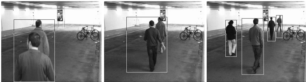
Fig. 22: Result of object tracking of 45 th , 123 rd and 266 th frame of video 7
