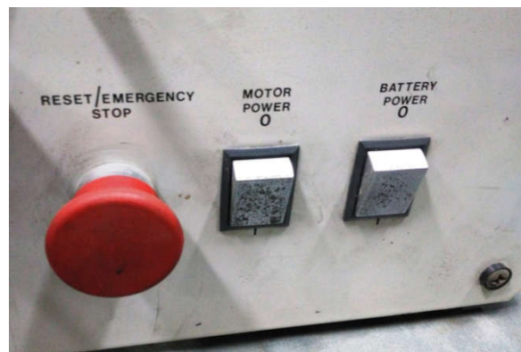
Fig. 2.15 Reset Button with motor power and battery power switch
