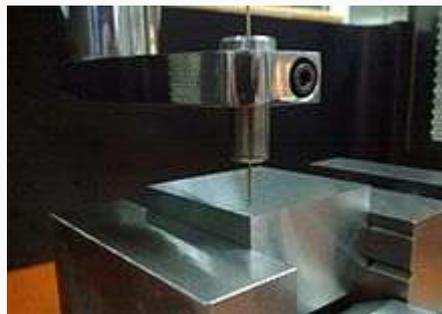
Fig1.3: Small hole drilling EDM machines.[27]
