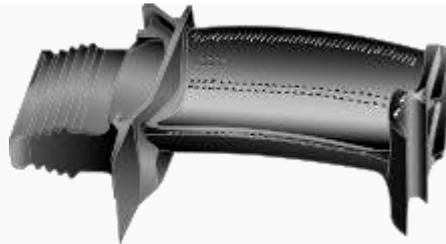
Fig1.2: A turbine blade with internal cooling as applied in the high-pressure turbine.[27]
