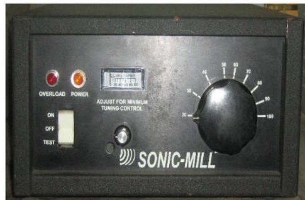
Fig. 2.3. Power supply & control unit
