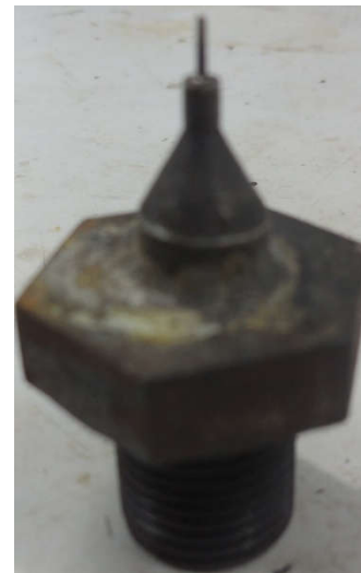
Fig. 2.7 Fabricated micro tool brazed with hexagonal bolt.
