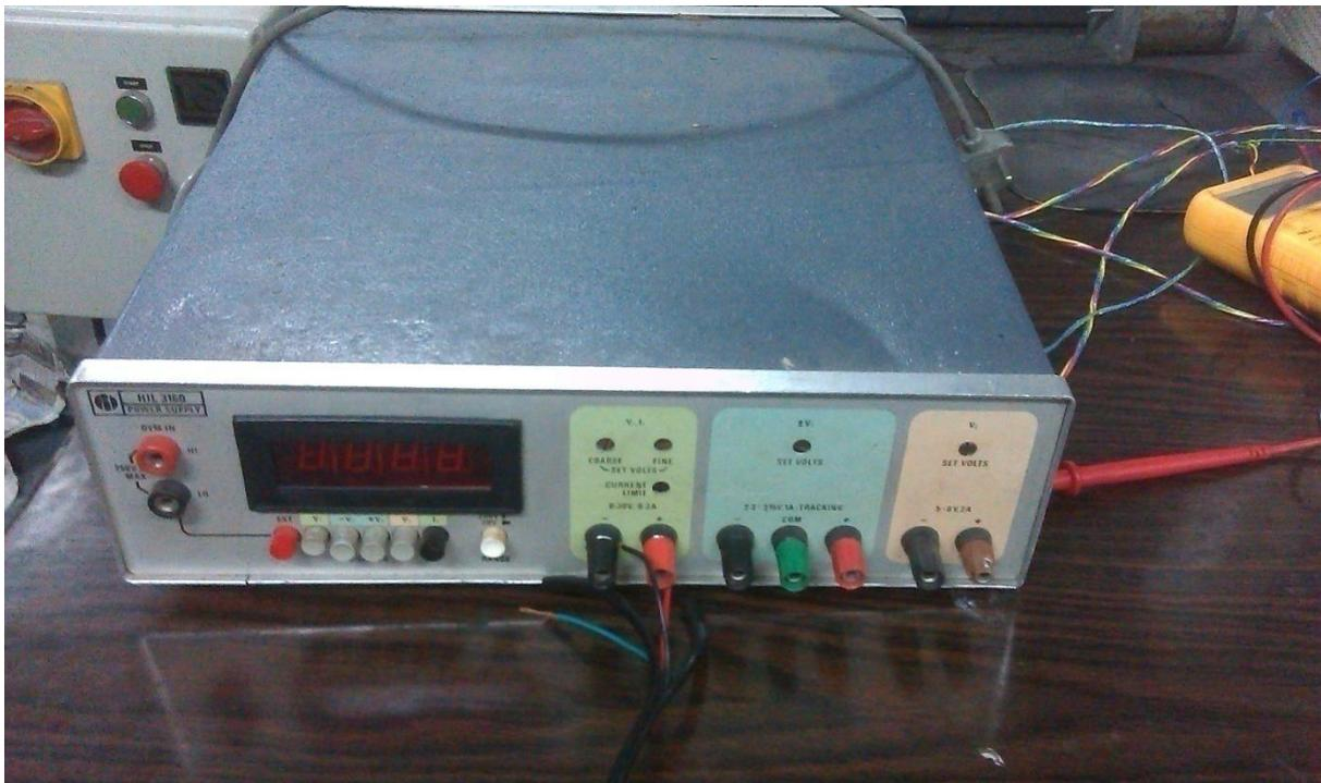
Fig: Photographic view of work piece rpm control unit
