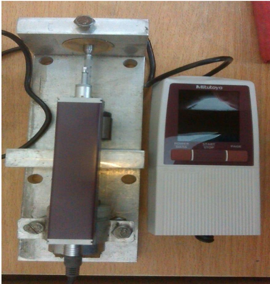
Fig: Photographic view of Mitutoyo Surface Roughness Tester
