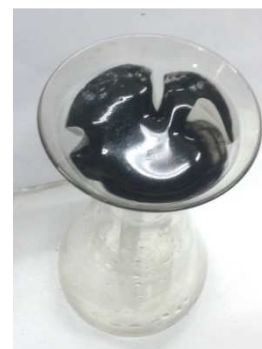
Fig8: filtration of conc slurry
