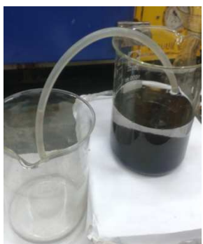
Fig5: upper layer discard by siphon
