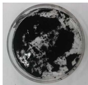
Fig11: catalyst after vacuum dried
