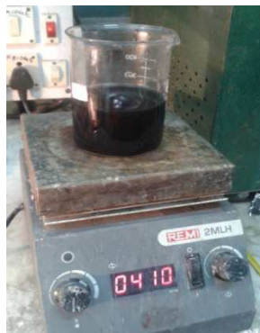
Fig2: Ag and Co salt added
