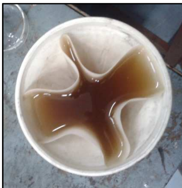
Fig 5: filtration of slurry GO
