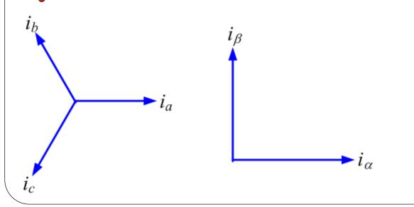
• Under this condition:  $|i_{\alpha}| = 1.5 |i_{a}|$   $|i_{\beta}| = 1.5 |i_{a}|$
