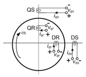
No torque is produced by interaction between flux and current that are on the same axis
