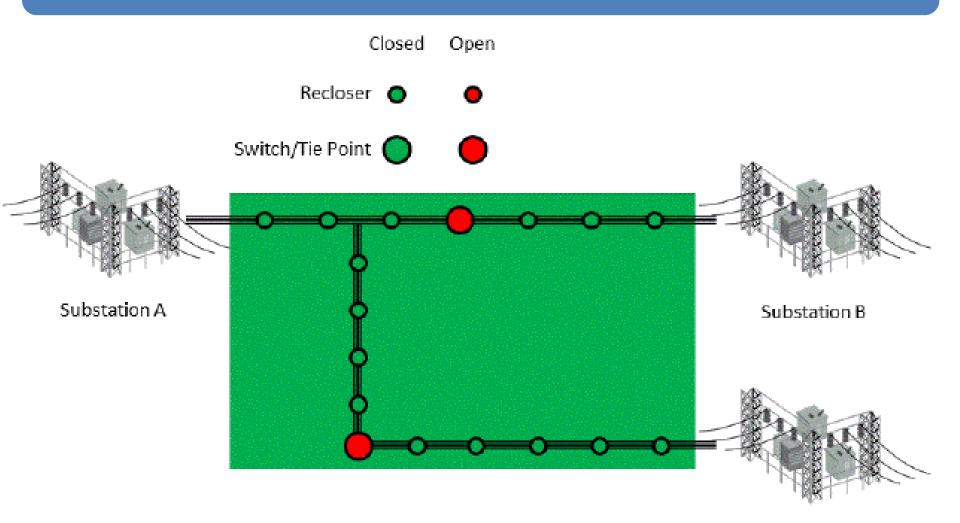
When a fault occurs, it causes all customers normally served by Substation A to lose power
