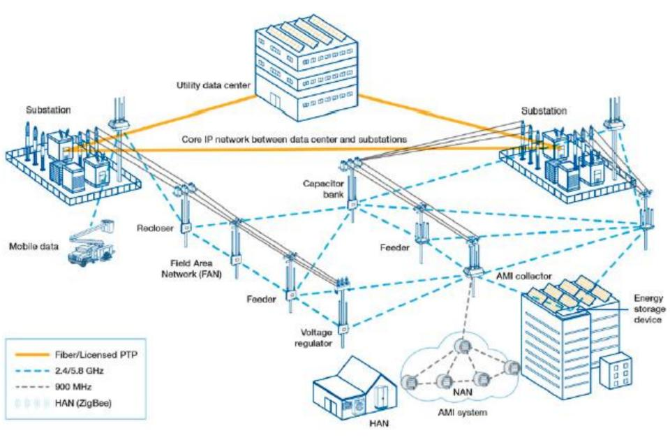
The OMS shares information with systems such as the GIS and IVR via the utility's enterprise network with workers and systems in the field using the FAN
