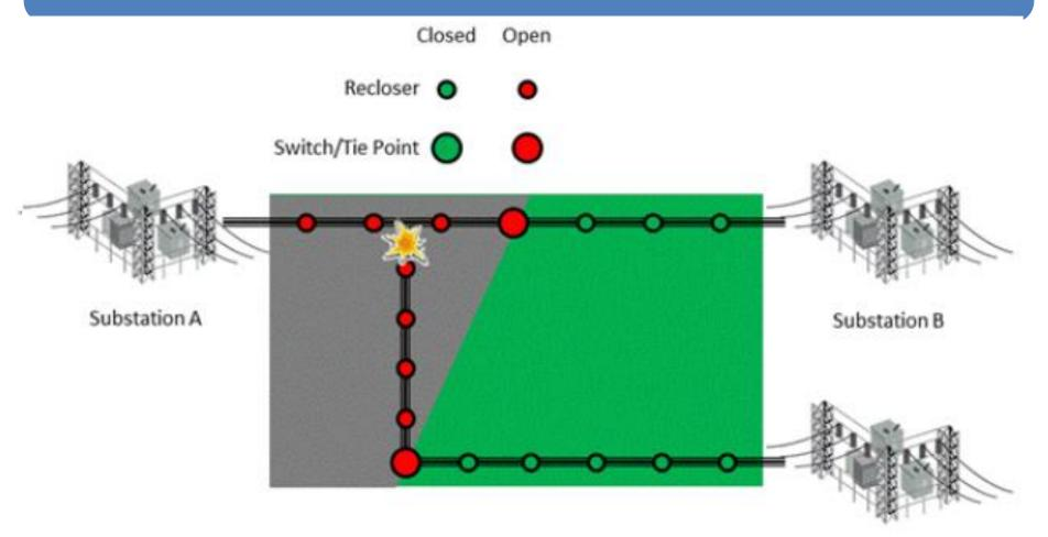
Now the outage is contained to the area between the accident site and the nearest recloser in the direction of each substation.
