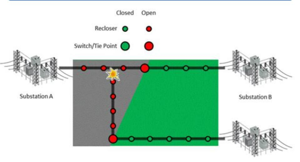
With smart reclosers and switches, service between the fault region and the various substations is restored by automatically closing the switches and the reclosers between the tie points and the fault
