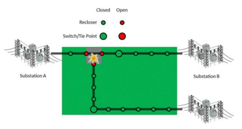
Without dynamic feeder reconfiguration, isolating the fault is a manual process
