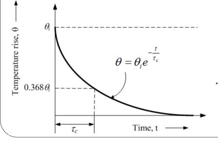
This is the cooling curve of a machine
