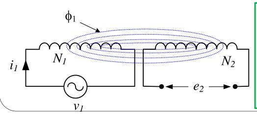
The action of mutual induction is reversible, i.e. any change in current in the second coil will also cause similar EMF to be induced in the first coil.
