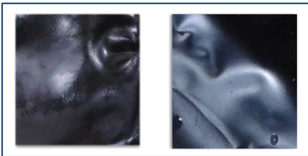
Fig. 4.1 (a) top (left) and bottom (right) surfaces of ABPBI membrane
