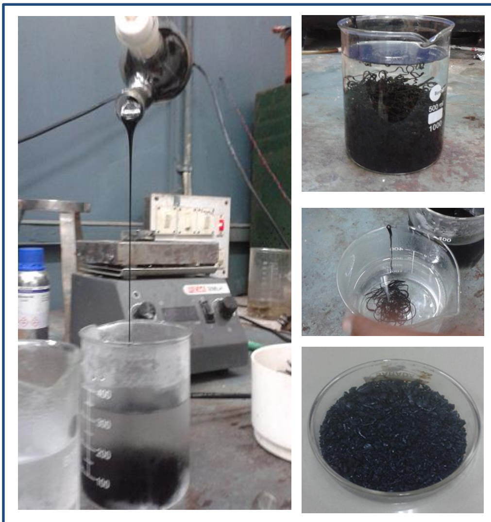
Fig 3.3.: (left) Polymerisation arrest by pouring polymer mixture into cold water. (right top and middle ) Thread like ABPBI polymer obtained. (right bottom) Cut and dried ABPBI polymer granules.
