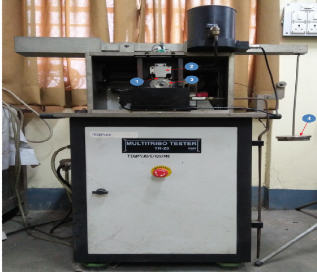
Figure 3.7(a) : Multi Tribotester Lever Load Mechanism
