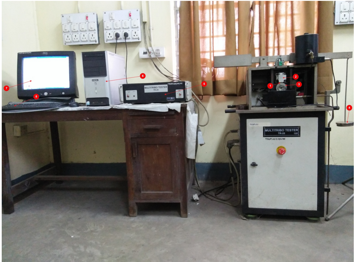
Figure 3.7 : Test setupBlock-on-roller configuration of Multi Tribotester “TR-25” (DUCOM, India) ”Tribometer”
