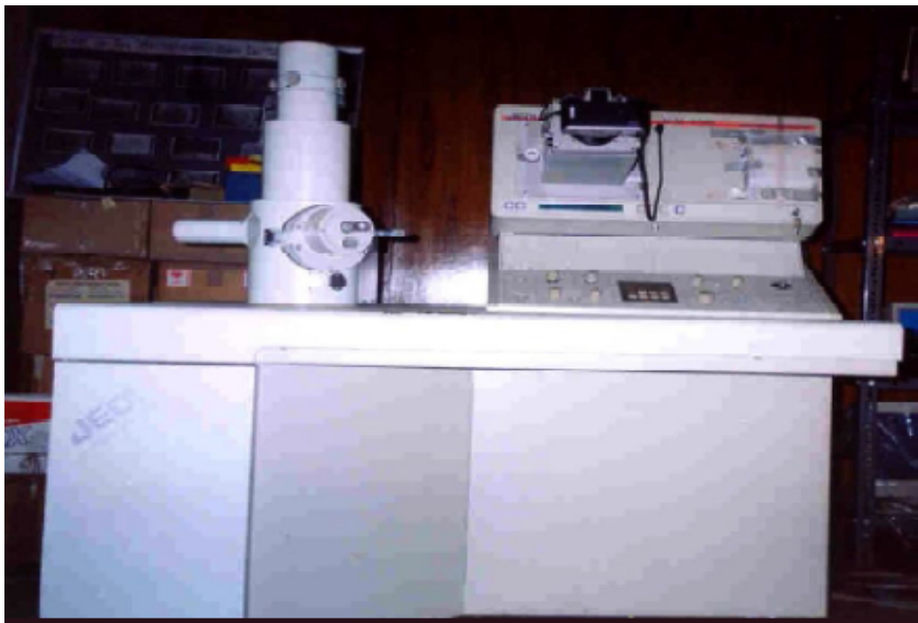
Fig 3.8 Photograph of the Scanning Electron Microscope (SEM) Machine used
