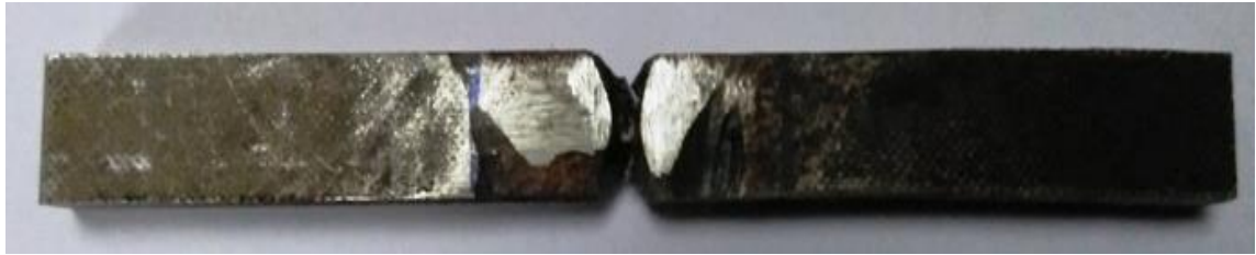
Figure 3.10(b) Photographic view of tensile test of notched specimen
