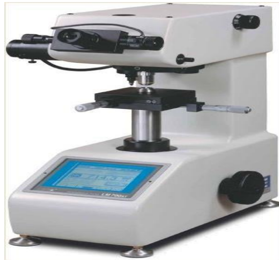
Figure 3.4 Photographic view of the Leco LM248AT micro-hardness tester
