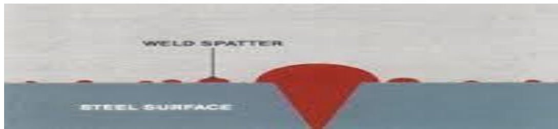
Figure 1.2(f) Spatter in welding [9]
