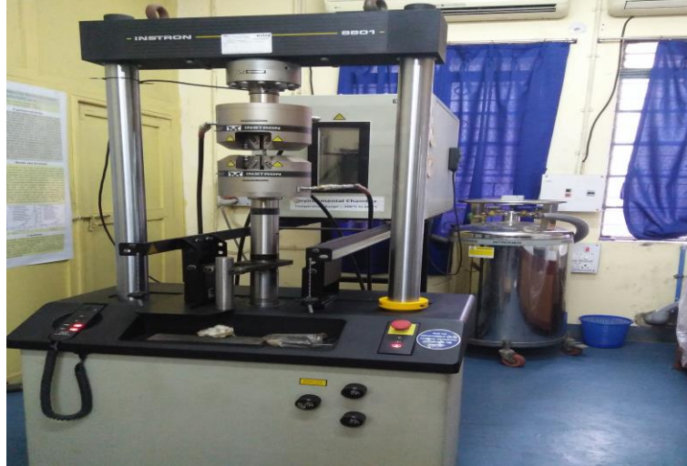
Figure 3.2 Photographic view of Instron universal testing machine
