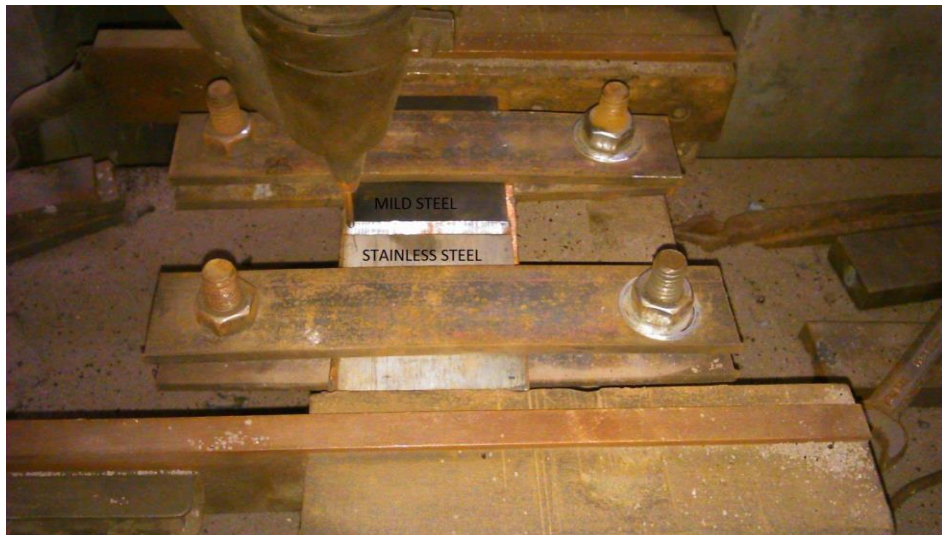
Figure 3.7 Welding set up
