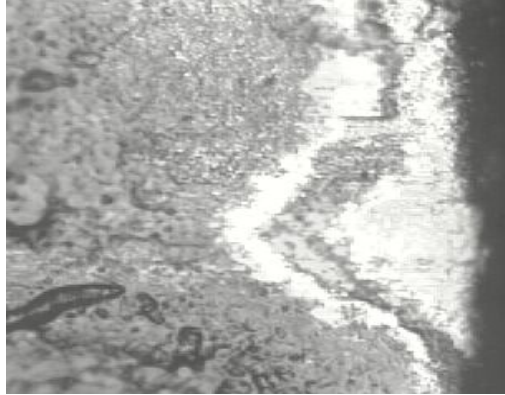
Fig. 4.1(u) The microscopic view of wear at cutting condition of at spindle speed 800 rpm, feed 0.08 mm/rev and depth of cut 1.2 mm
