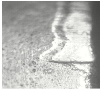
Fig. 4.1(q) The microscopic view of wear at cutting condition of at spindle speed 800 rpm, feed 0.08 mm/rev and depth of cut 1.0 mm
