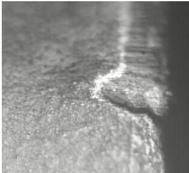
Fig. 4.3(o) Microscopic view of wear at cutting condition of at spindle speed 620 rpm, feed 0.08 mm/rev and depth of cut 1.0 mm
