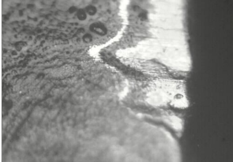
Fig. 4.2(u) The microscopic view of wear at cutting condition of at spindle speed 800 rpm, feed 0.08 mm/rev and depth of cut 1.2 mm
