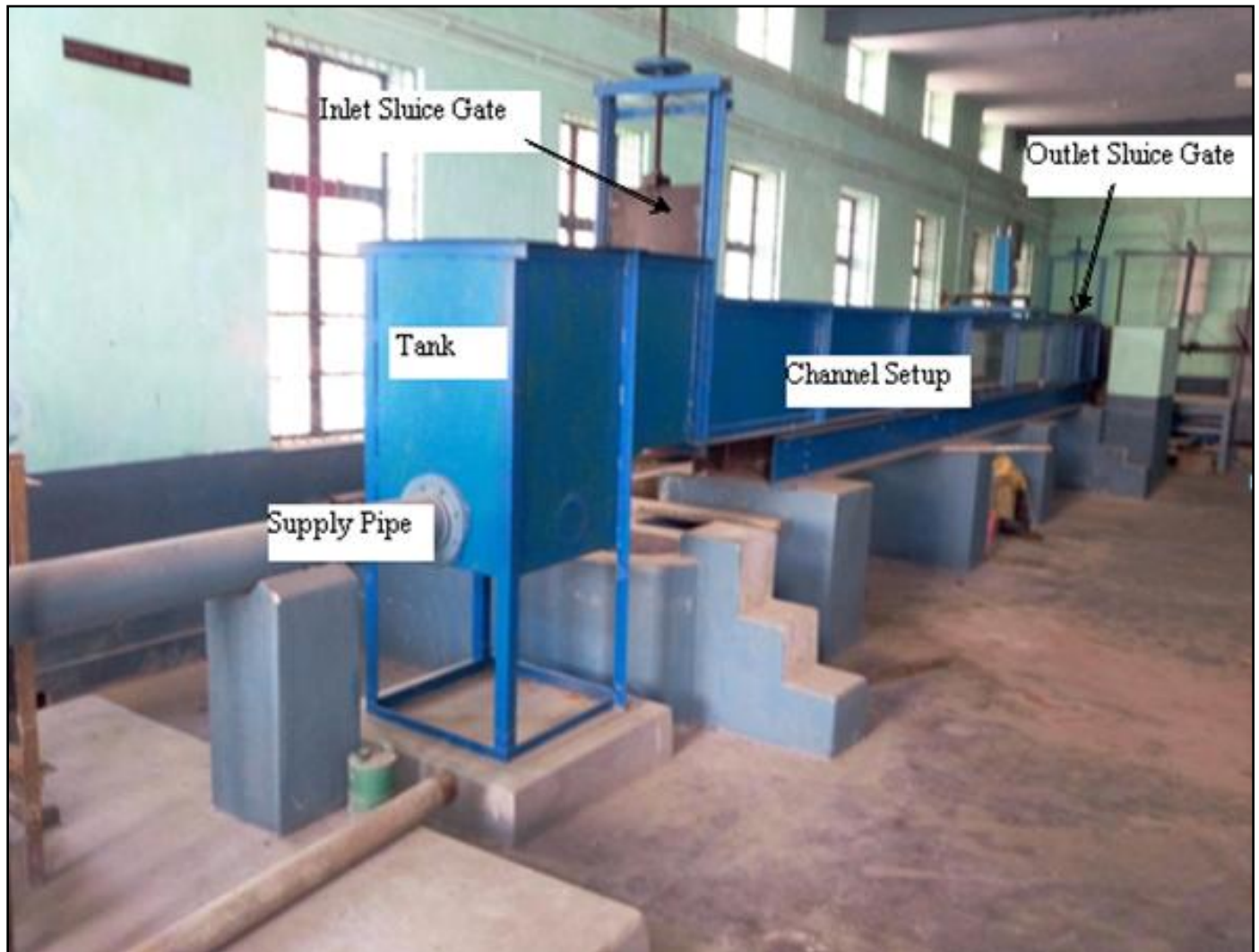
Fig 3.1.1, Rectangular Channel Setup
