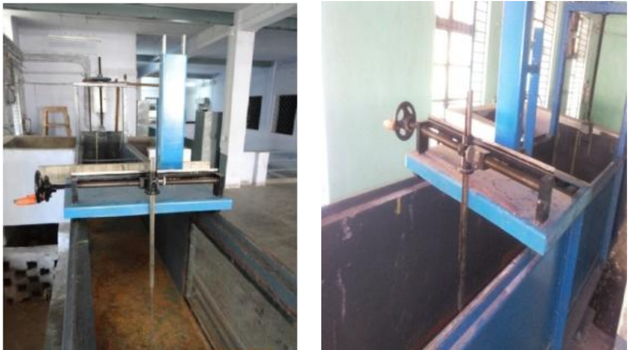
Fig 3.1.3, Point gauge mounted on moving trolley
