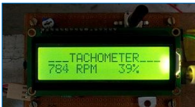
Fig.5.43: Tachometer showing critical speed Fig.5.44: Strain data on phone via Bluetooth
