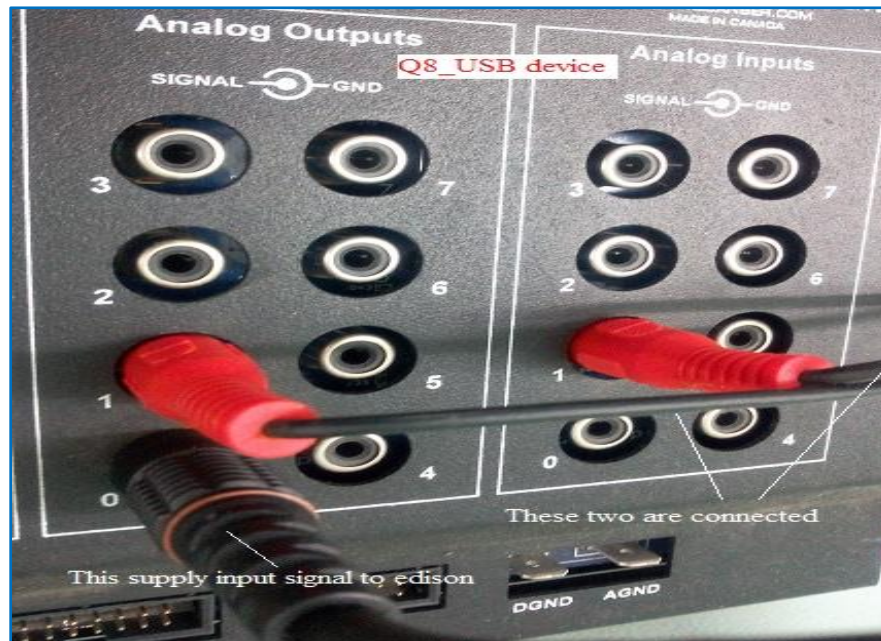
Fig.2.6: Connections of Q8_USB
