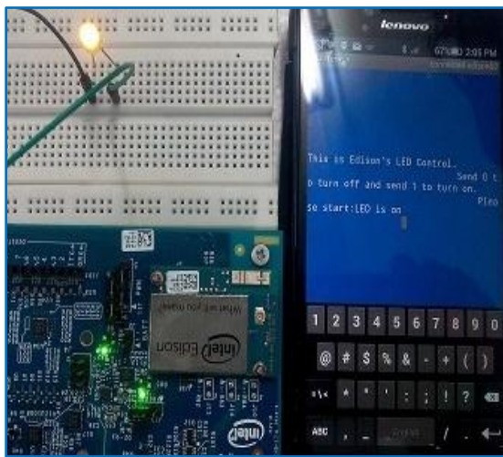
Fig.3.6: Turning LED on by sending command '1' over Bluetooth.
