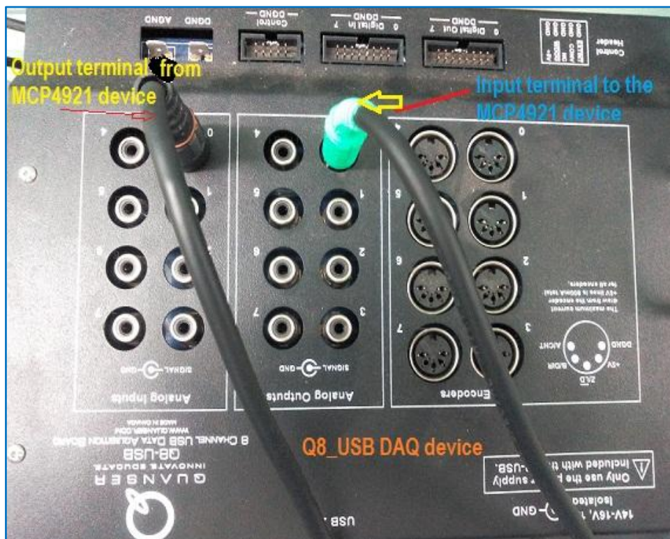
Fig.4.7: The DAQ device, connected to two terminals
