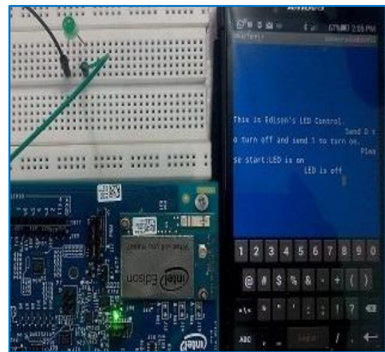
Fig.3.7: Turning LED off by sending command '0' over Bluetooth.
