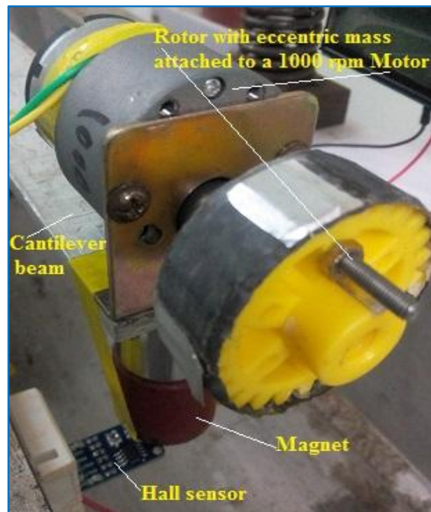
Fig.5.2: Actuation system for inducing vibration
