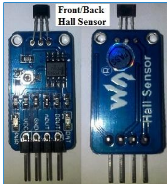
Fig.5.4 Hall sensor used in experiment
