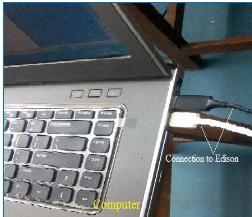
Fig.2.4: Two USB serial ports connected between computer and Edison
