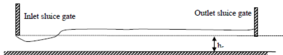
Fig 5.1: A simple sketch of free hydraulic jump when inlet sluice gate and outlet sluice gate are at critical depth
