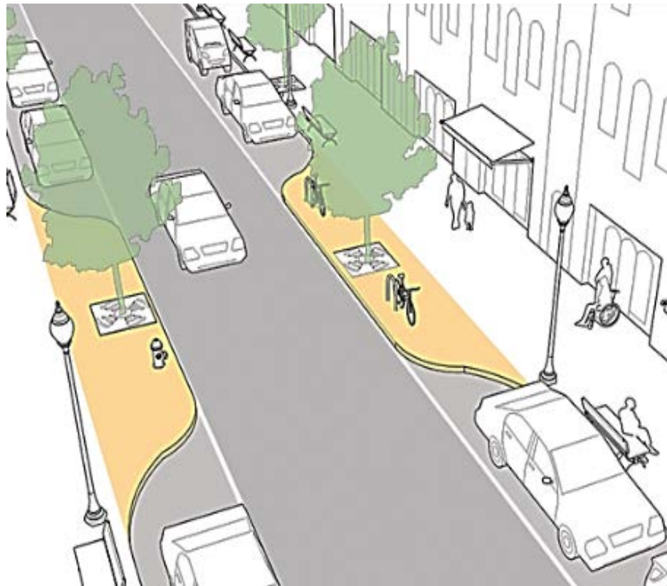
Fig 7.5 Bus bulb and Pinch Point
