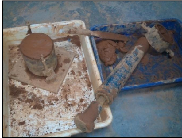
Fig-7.10: Proctor Test Experimental Setup
