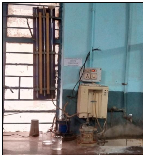
Fig-7.9: Falling Head Permeability Apparatus Setup used in the Experiment
