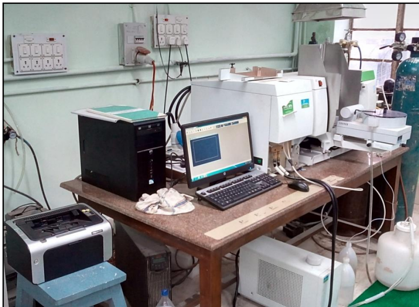
Fig-7.22: PerkinElmer (AAAnalyst400) Atomic Absorption Spectrophotometer (AAS)
