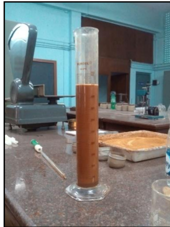
Fig-7.18: Grain Size Distribution Experimental Setup
