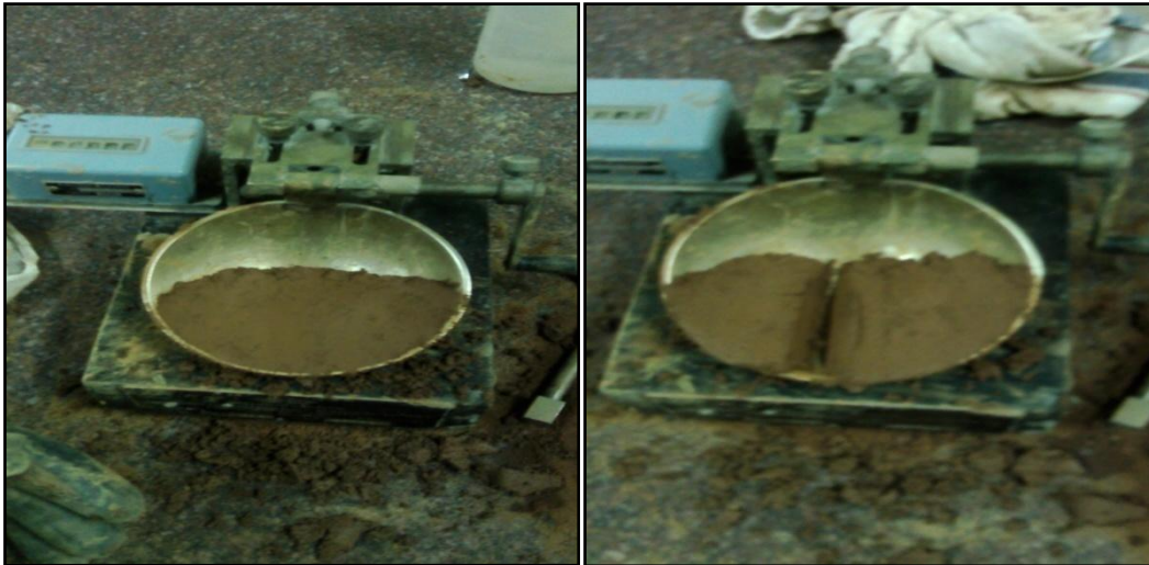
Fig-7.1: Before Application of Blows
