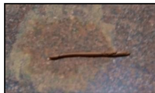
Fig-7.4: Rolling Up of the Sample into Thread while Determining Plastic Limit
