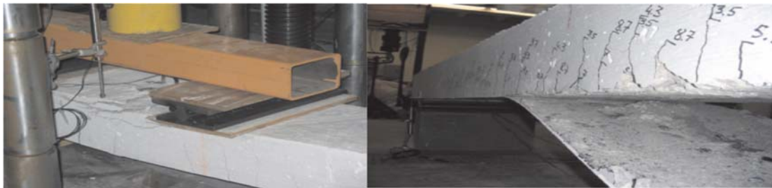
Figure 2.5: photograph of failed specimen control specimen and externally bounded FRP specimen
