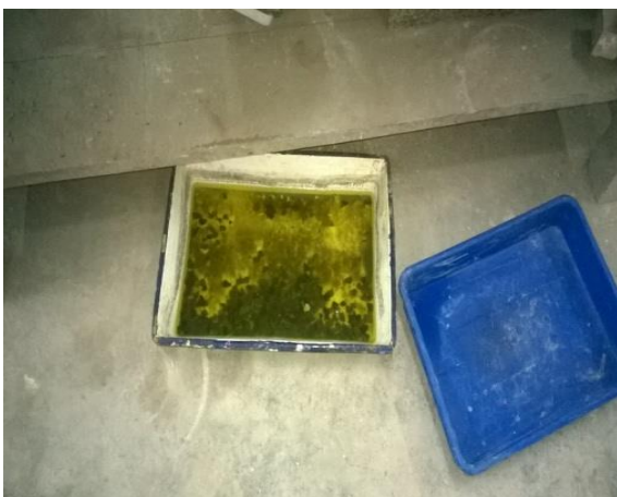
Fig 3.4: Recycled aggregate on Hcl solution Fig3.5: Remove out recycled aggregate from Hcl solution after 48 hours
