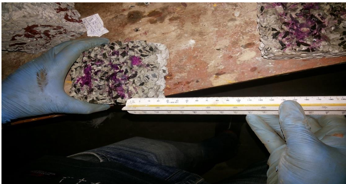
Fig4.13: Measurement of depth of carbonation in porous concrete cube after 30 days of carbonation chamber
