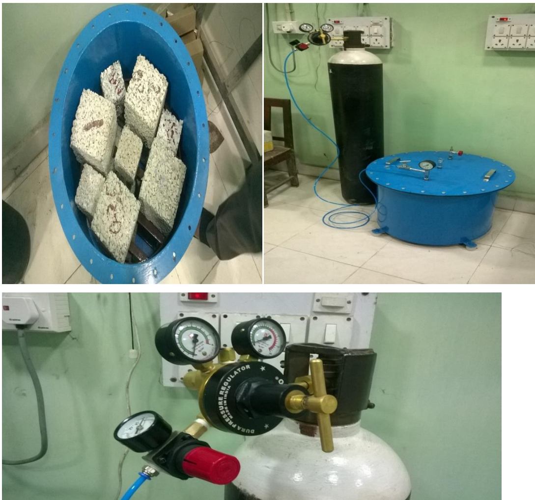
Fig 3.14: carbonation test set up in carbonation chamber
