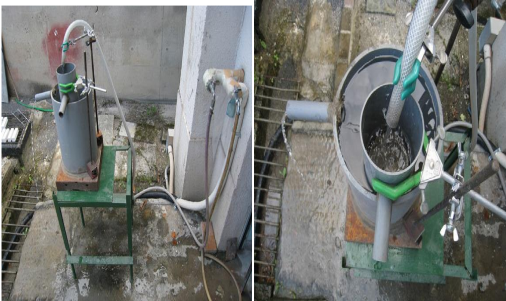
Fig2.1.17. Water permeability set-up for porous concrete.
