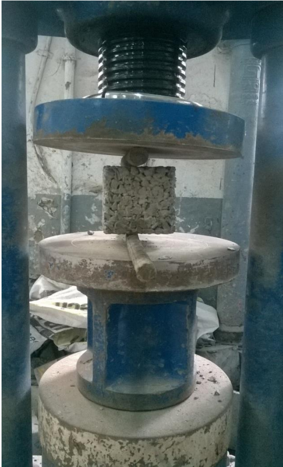
Fig 3.16: Breaking of concrete cube sample in equal parts & applying phenolphthalein indicator on fracture concrete cube and cylinder surface
