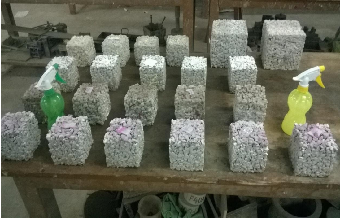
Fig 3.15: phenolphthalein indicator applied on porous concrete cube
