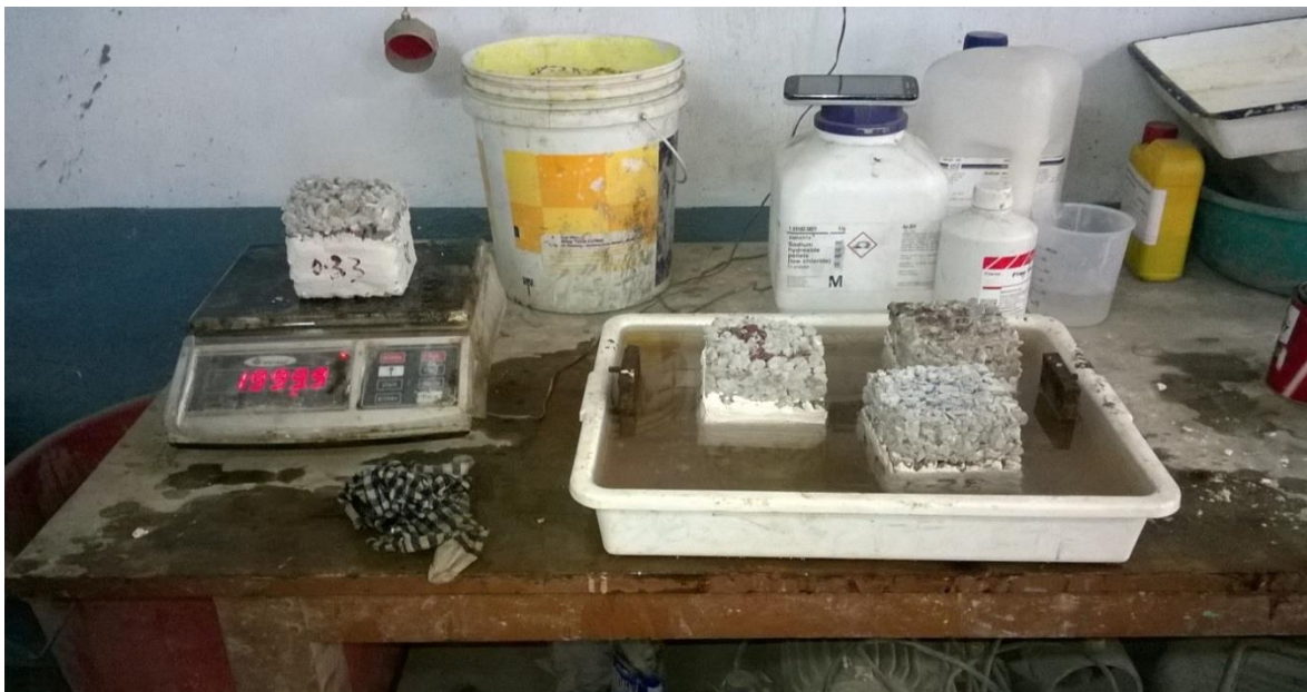
Fig 3.6 Sorptivity test of cube sample
