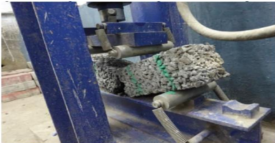
Fig. 3.13: Failure of prism Specimen after loading
