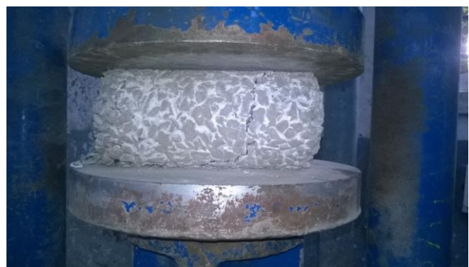
Fig 3.11: Crack in cylindrical specimen after tensile load is applying
