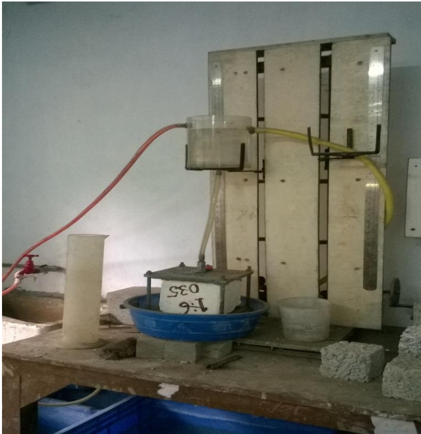
Fig 3.8: Constant head permeability test set up
