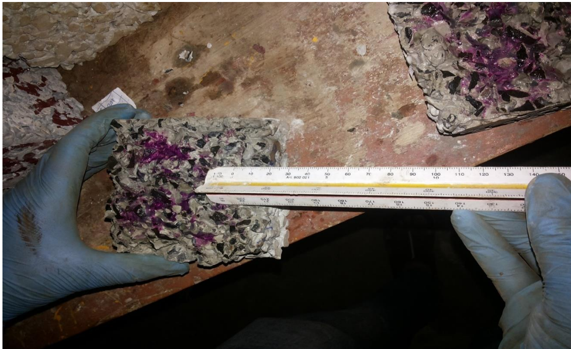
Fig4.12: Measurement of Depth of carbonation in porous concrete cube after 10 days of carbonation chamber
