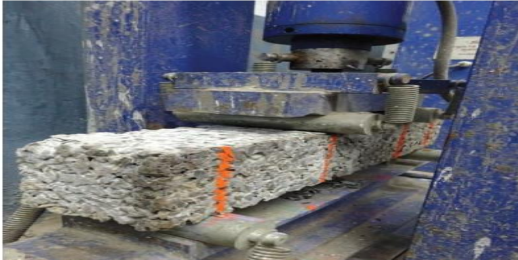
Fig. 3.12: Arrangement for loading of flexural test specimen
