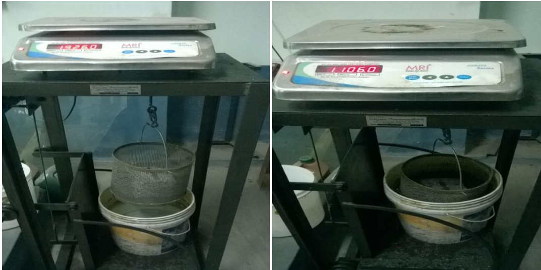
Fig 3.7: Submerged weight of porous concrete cube for porosity test
