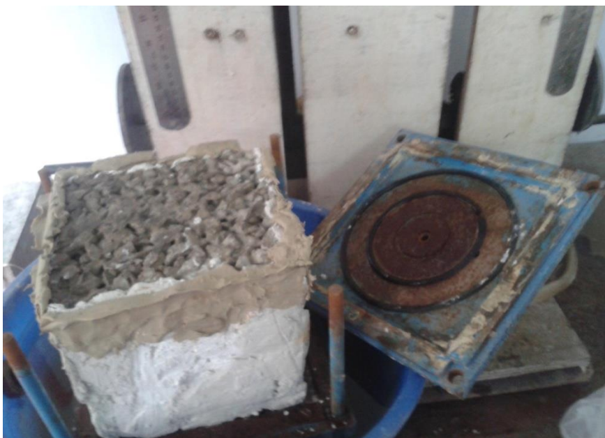
Fig 3.9: Putty to prevent leakage in transverse direction
