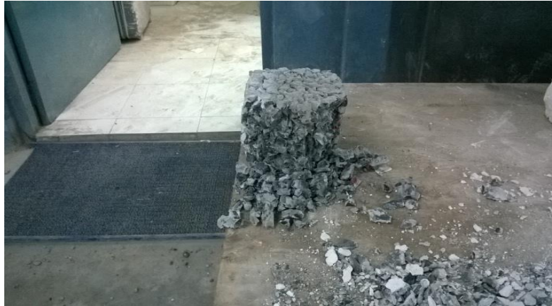
Fig 3.10: The failure of cube specimen after testing
