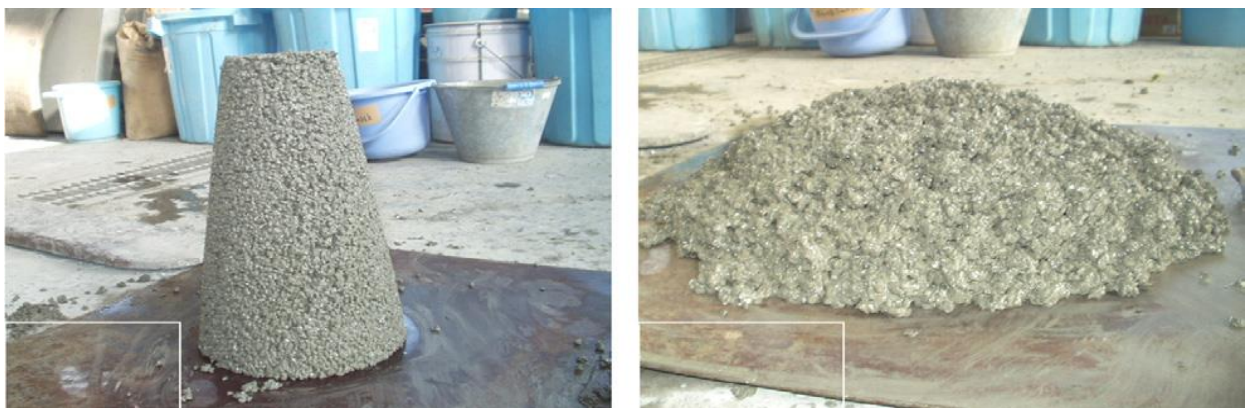
Fig.2.1. 13. Slump and slump-flow of CPC and HPPC.
