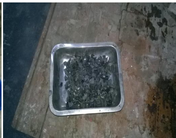
Fig 3.4: Recycled aggregate on Hcl solution Fig3.5: Remove out recycled aggregate from Hcl solution after 48 hours
