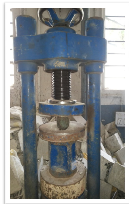
Fig-3.3.4 Split tensile strength testing
