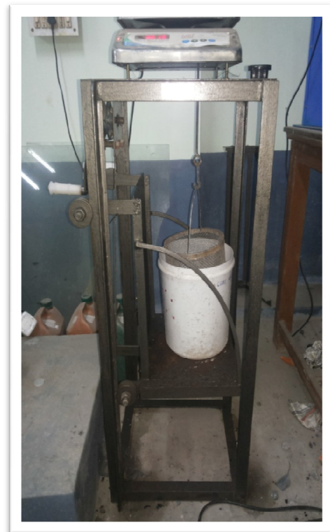
Fig.3.3.2. Arrangement to measure Apparent Porosity
