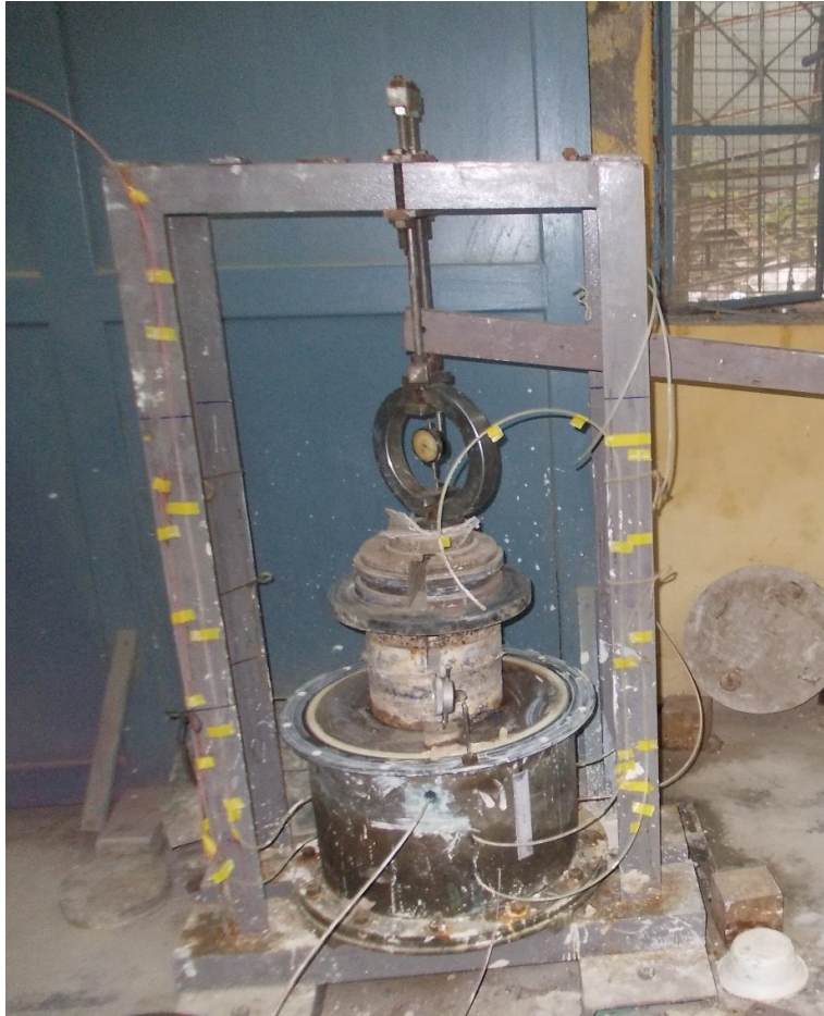
Fig 5.3: Photograph of Consolidation Tank
