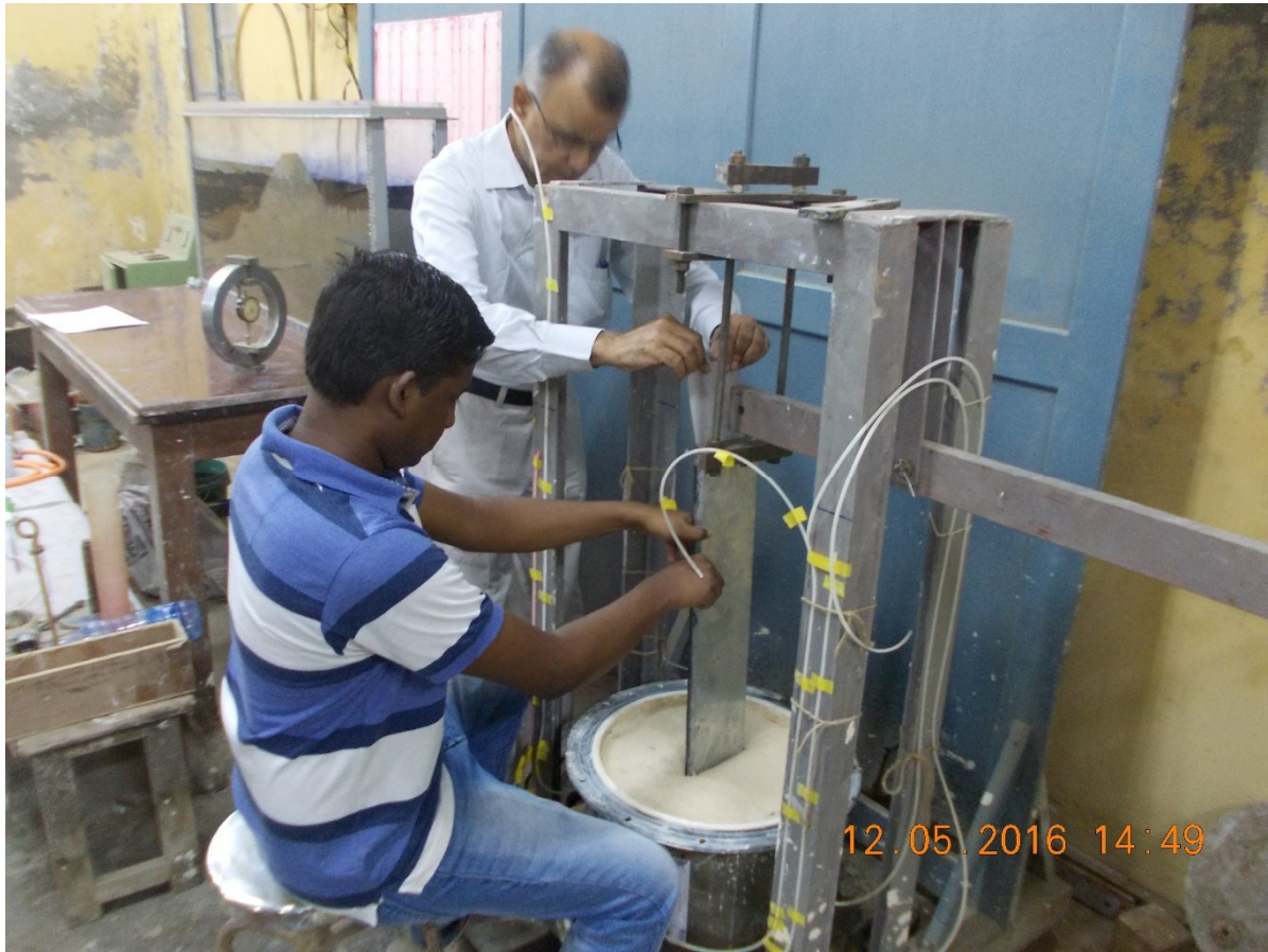
Fig 5.4: Installation Of Pre-fabricated Vertical Drain
