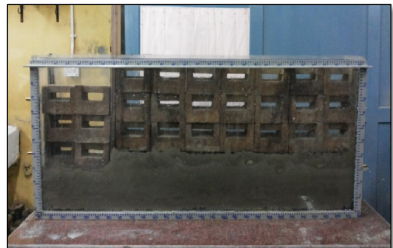
Figure 6.6 – Stage-2, Construction of Berm
