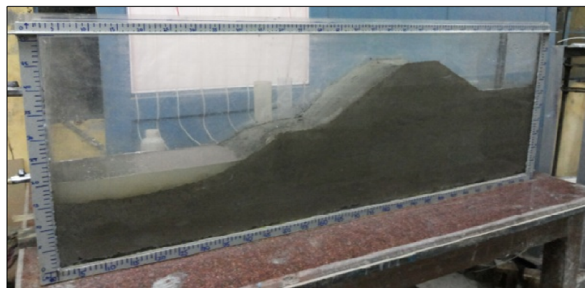
Figure 6.9 – 3D view of completed embankment showing river side and land side
