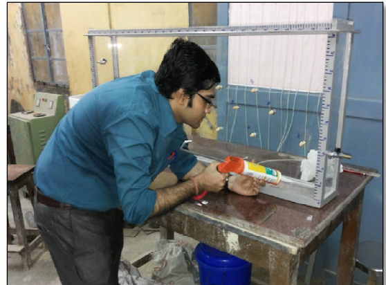
Figure 6.4 – Waterproofing of tank
