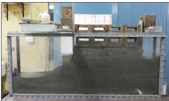
Figure 6.7 –Stage-3, Construction of Embankment
