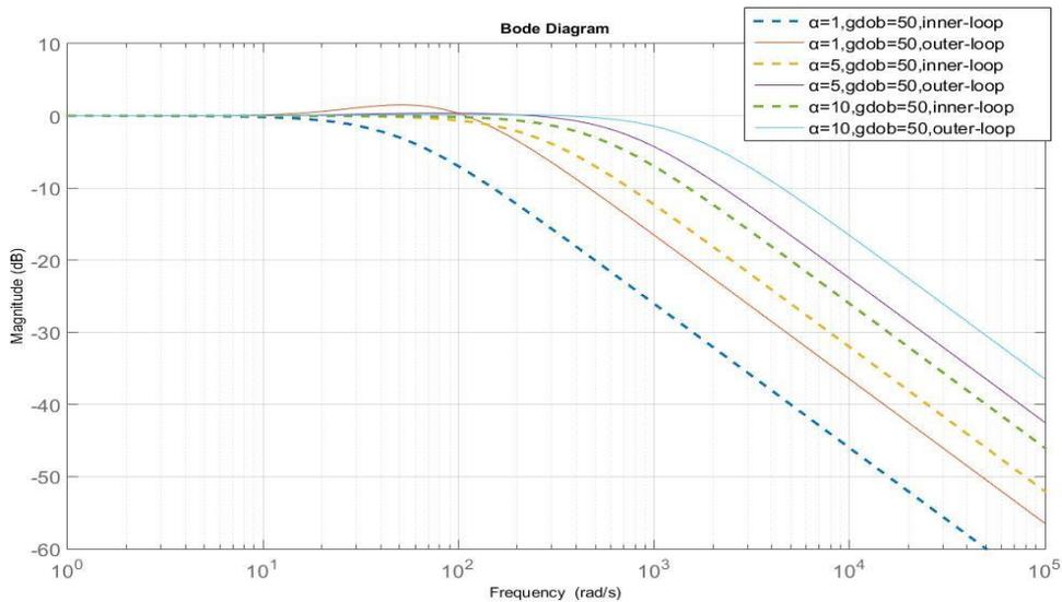
Fig. 4.13- Inner loop and outer-loop Co-sensitivity function frequency responses
