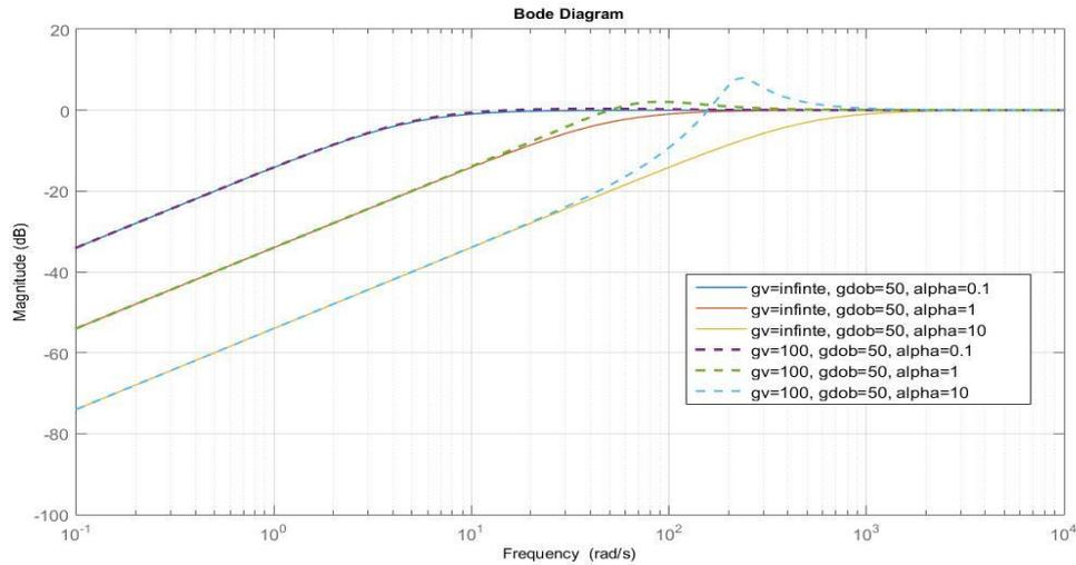
Fig. 4.7- Sensitivity function for different values of  $\alpha$
