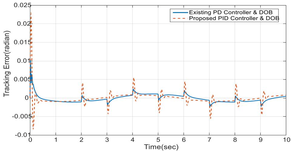
Fig.6.17-Tracking Error of the system for sinusoidal input and square disturbance applied at t=0 and t=2 respectively
