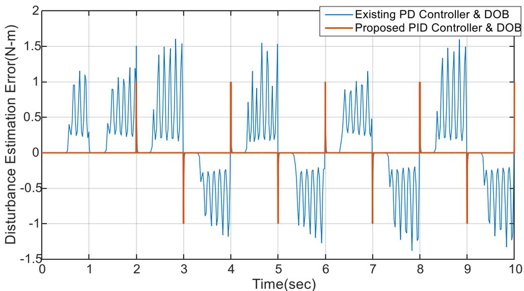
Fig.6.5- Disturbance estimation error when square input as position reference and square disturbance is applied at t=0 and t=2 sec respectively
