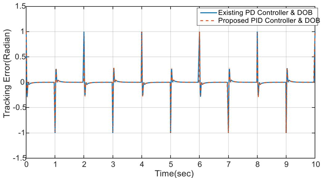
Fig.6.14a- Tracking error when square input as position reference and sinusoidal disturbance is applied at  $t=0$  and  $t=2$  sec respectively
