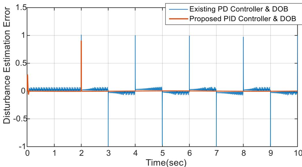
Fig.6.10- Disturbance Estimation Error of the system for sinusoidal input and square disturbance applied at  $t=0$  and  $t=2$  respectively
