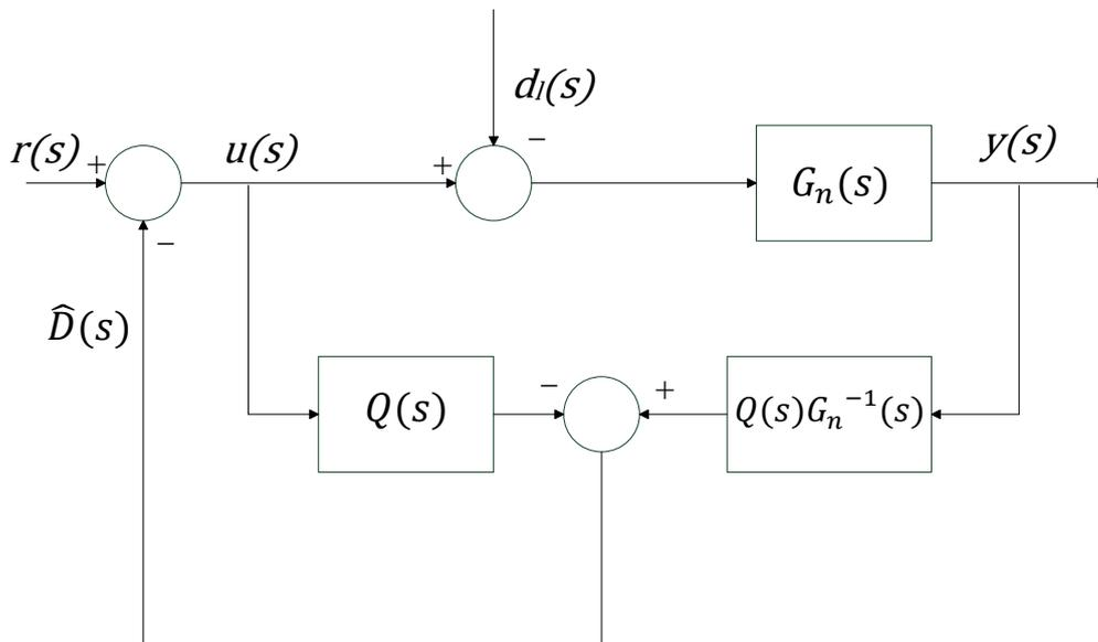
Fig. 3.3b- Block diagram of a frequency domain DOB for minimum phase linear system, an equivalent form [26]
