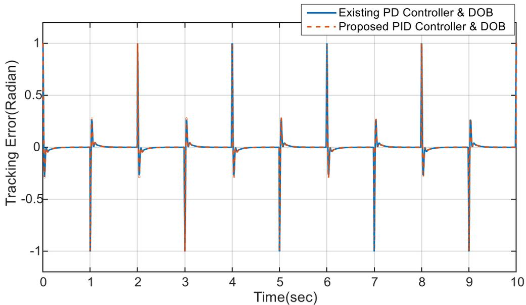
Fig.6.15a- Tracking error when square input as position reference and square disturbance is applied at  $t=0$  and  $t=2$  sec respectively
