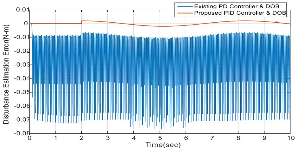
Fig.6.2- Disturbance estimation error when sinusoidal input as position reference and sinusoidal disturbance is applied at  $t=0$  and  $t=2$  sec respectively
