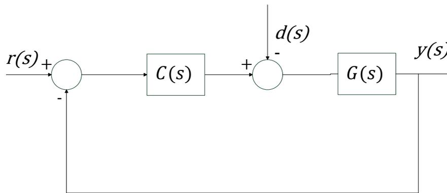
Fig. 3.2- Block diagram of a basic feedback control system
