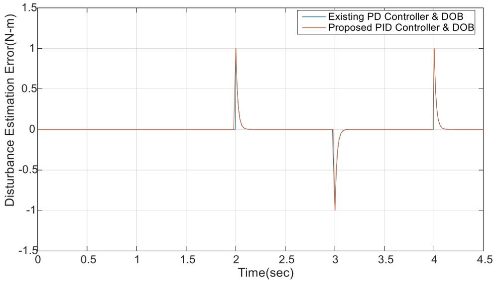
Fig.6.4b- Disturbance estimation error when sinusoidal input as position reference and square disturbance is applied at t=0 and t=2 sec respectively (zoomed up to 4.5 seconds)
