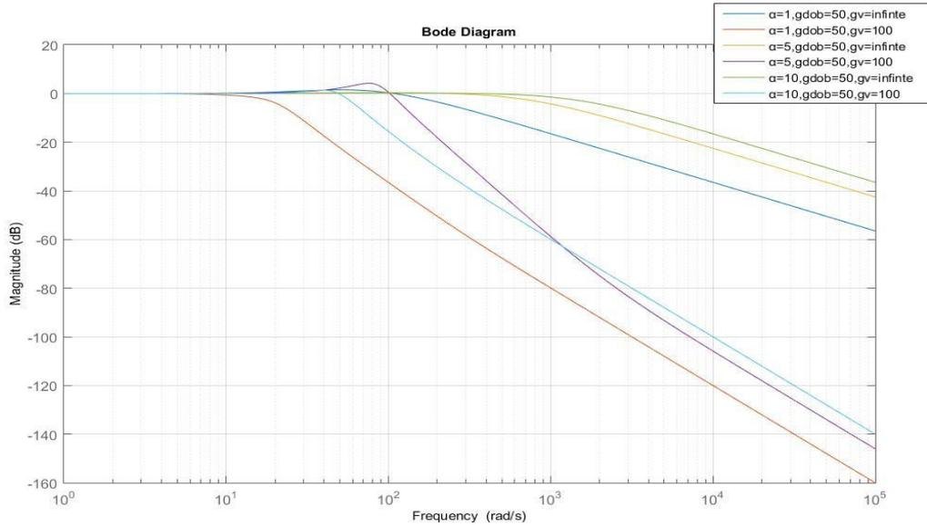
Fig. 4.12- Outer-loop Co-Sensitivity function frequency responses for different values of  $\alpha$
