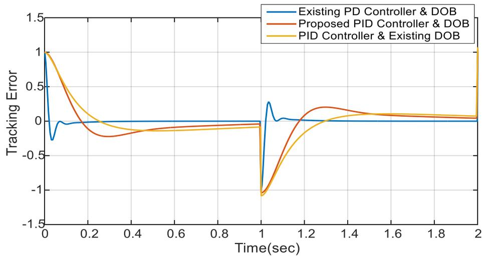
Fig.6.21b-Tracking Error of the system for square input and square disturbance applied at  $t=0$  and  $t=1.5$  respectively (zoomed up to 2 seconds)
