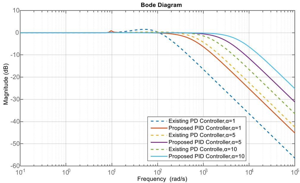
Fig.5.10- Comparison of Co-sensitivity function frequency response for outer-loop
