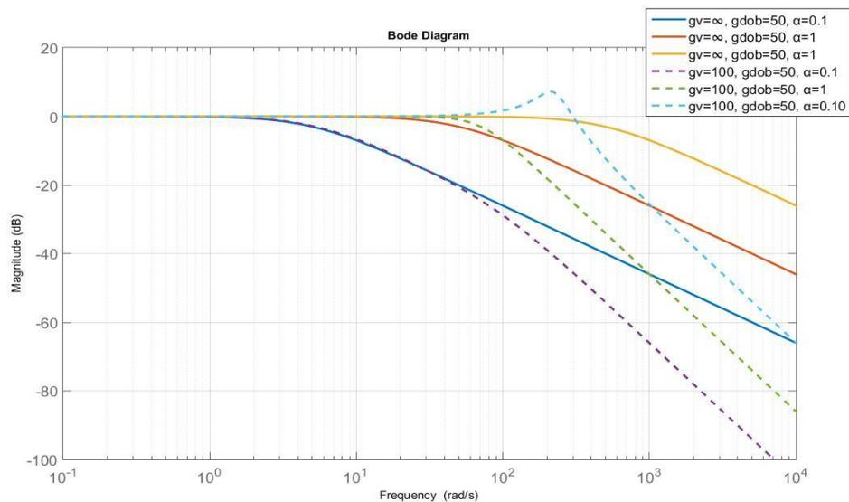
Fig. 4.8- Co-Sensitivity function for different values of  $\alpha$
