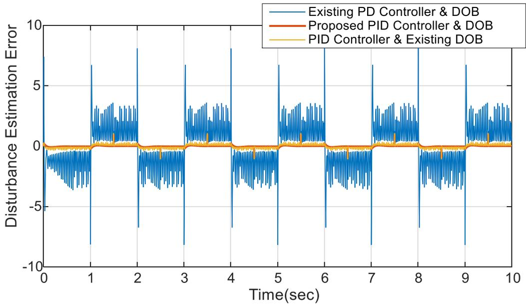
Fig.6.11a- Disturbance Estimation Error of the system for square input and square disturbance applied at  $t=0$  and  $t=1.5$  respectively
