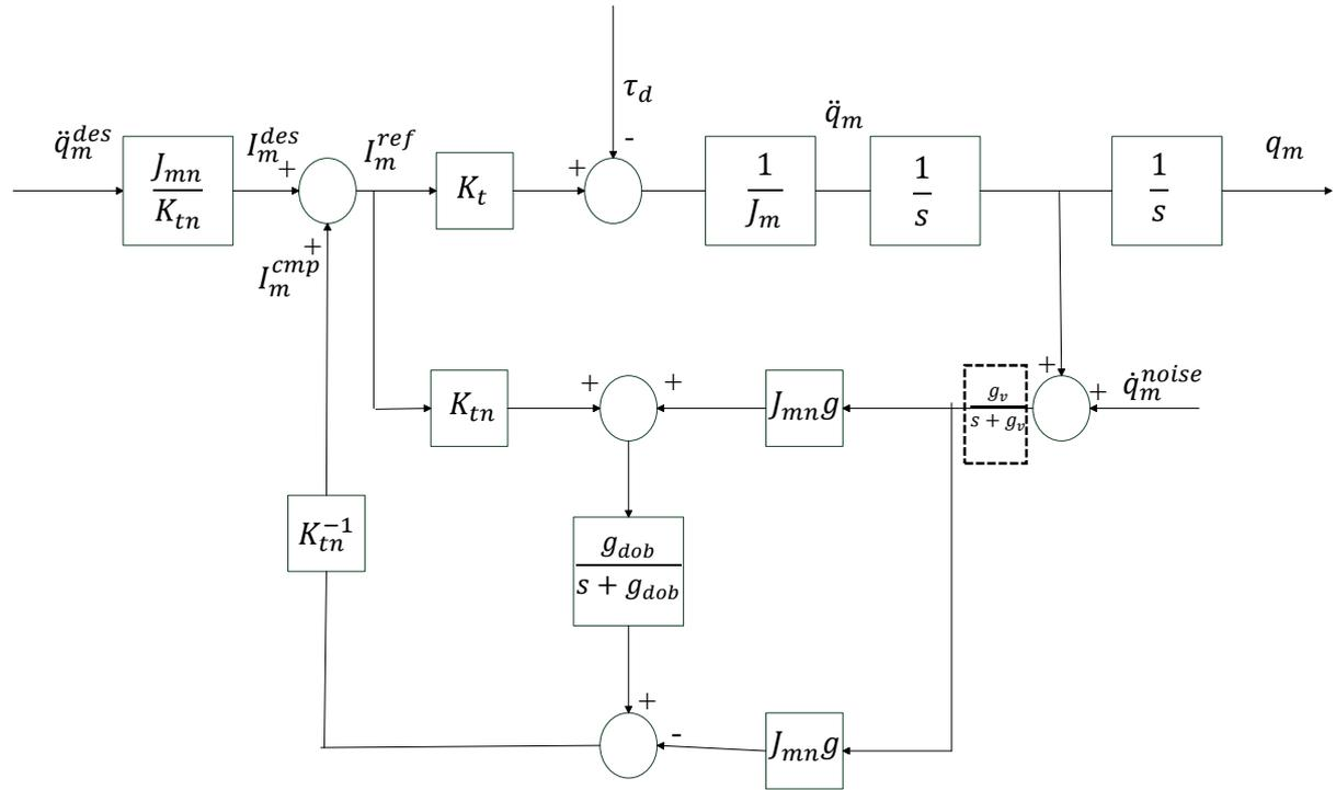
Fig. 4.4- Block diagram of a DOB based motion control system considering ideal velocity estimation, dotted transfer function is considered for practical velocity estimation [24]
