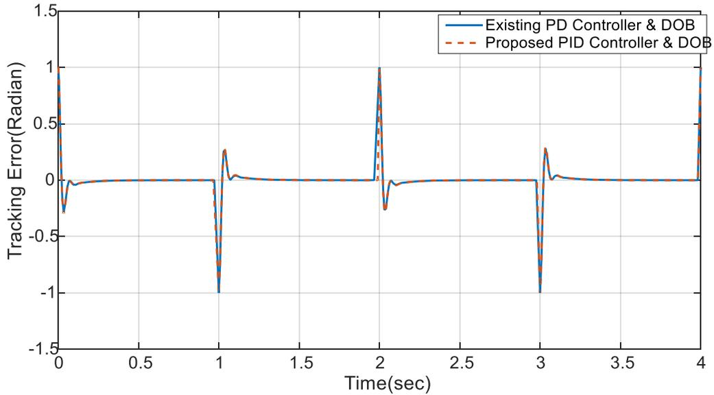
Fig.6.14b- Tracking error when square input as position reference and sinusoidal disturbance is applied at  $t=0$  and  $t=2$  sec respectively (zoomed up to 4 seconds)
