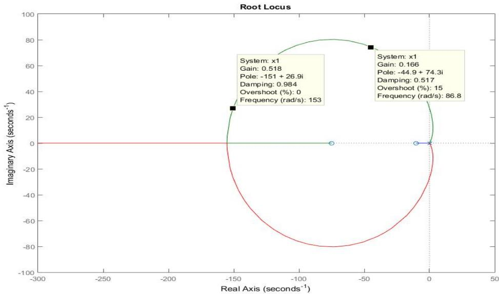
Fig. 4.14- Root locus plot showing stability of position control system
