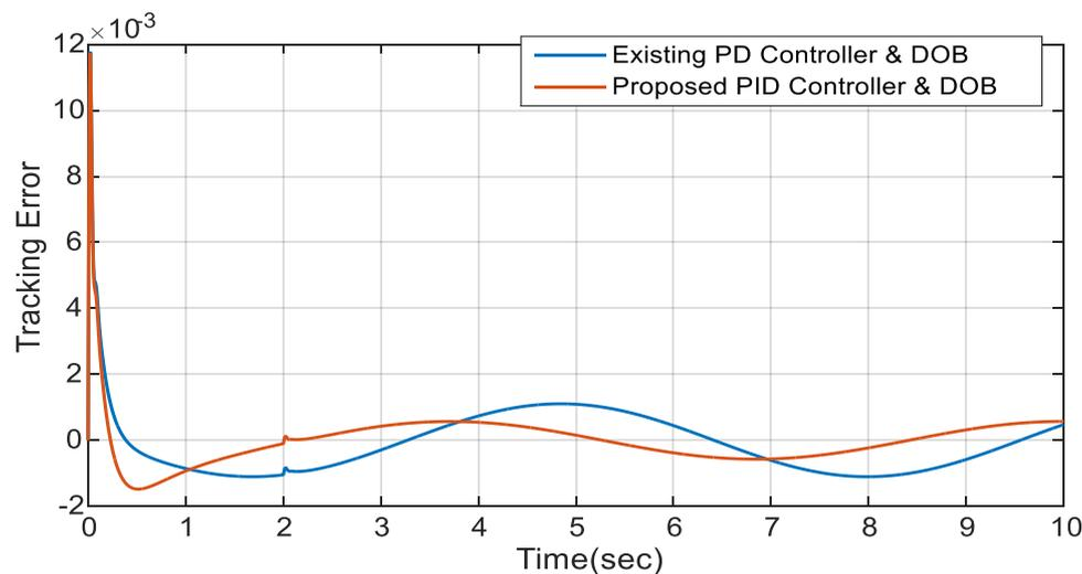
Fig.6.18- Tracking Error of the system for sinusoidal input and sinusoidal disturbance applied at t=0 and t=2 respectively
