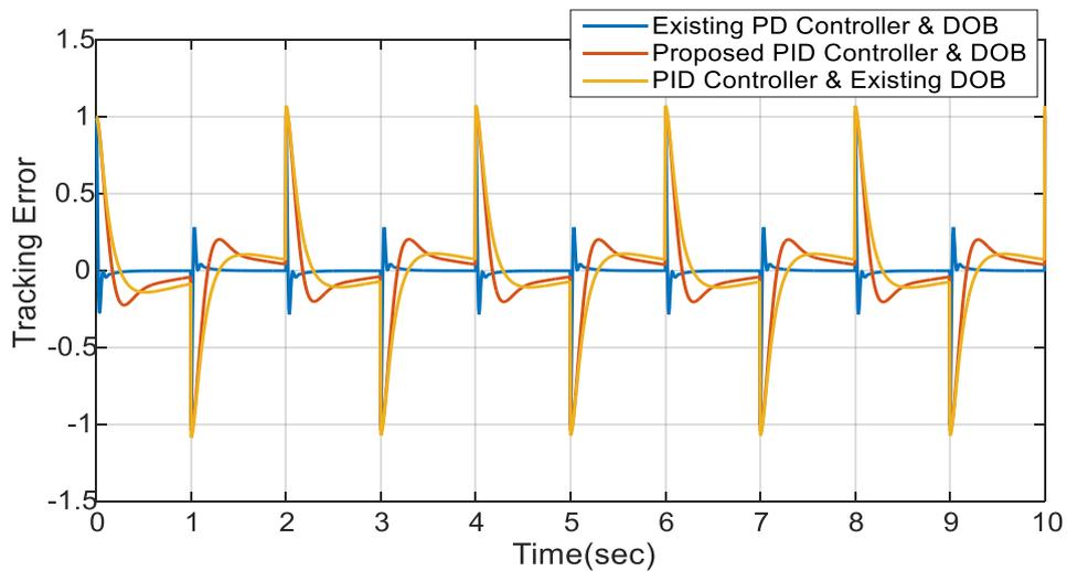
Fig.6.21a- Tracking Error of the system for square input and square disturbance applied at  $t=0$  and  $t=1.5$  respectively
