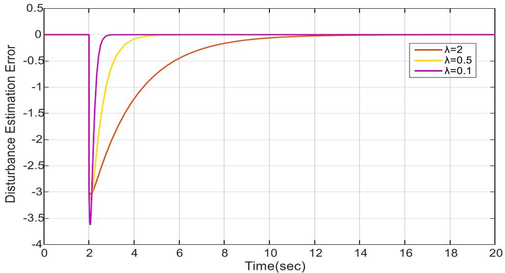
Fig.3.11- Disturbance estimation error plots for different  $\lambda$  values
