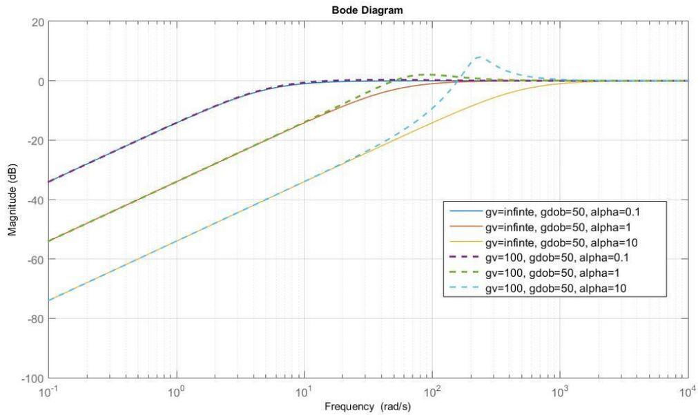
Fig. 5.2- Sensitivity function frequency responses for different values of  $\alpha$
