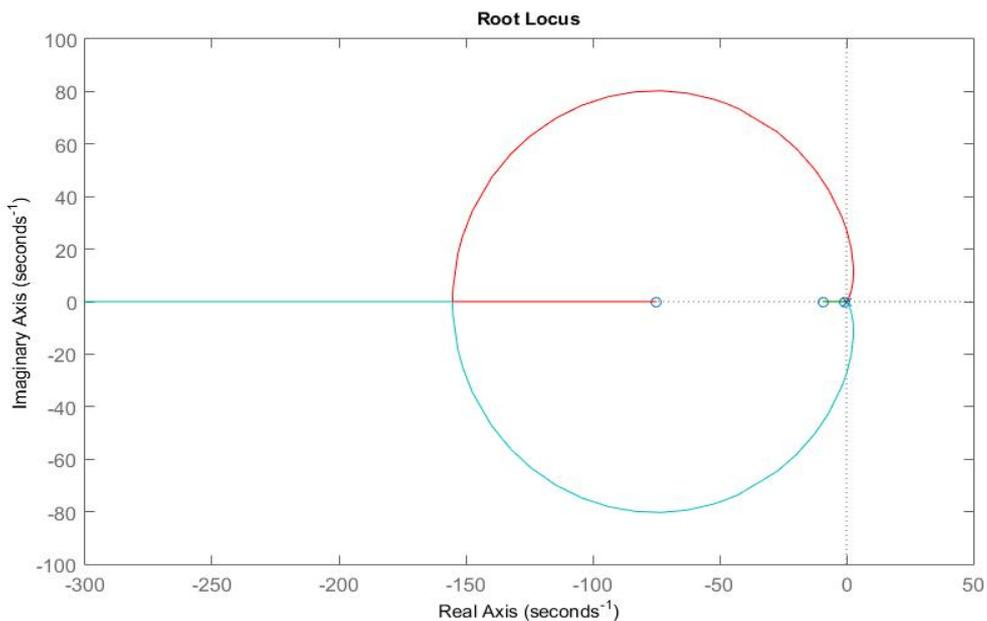
Fig. 5.11- Root locus plot for stability analysis
