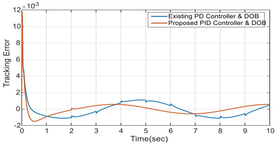
Fig.6.20- Tracking Error of the system for sinusoidal input and square disturbance applied at  $t=0$  and  $t=2$  respectively
