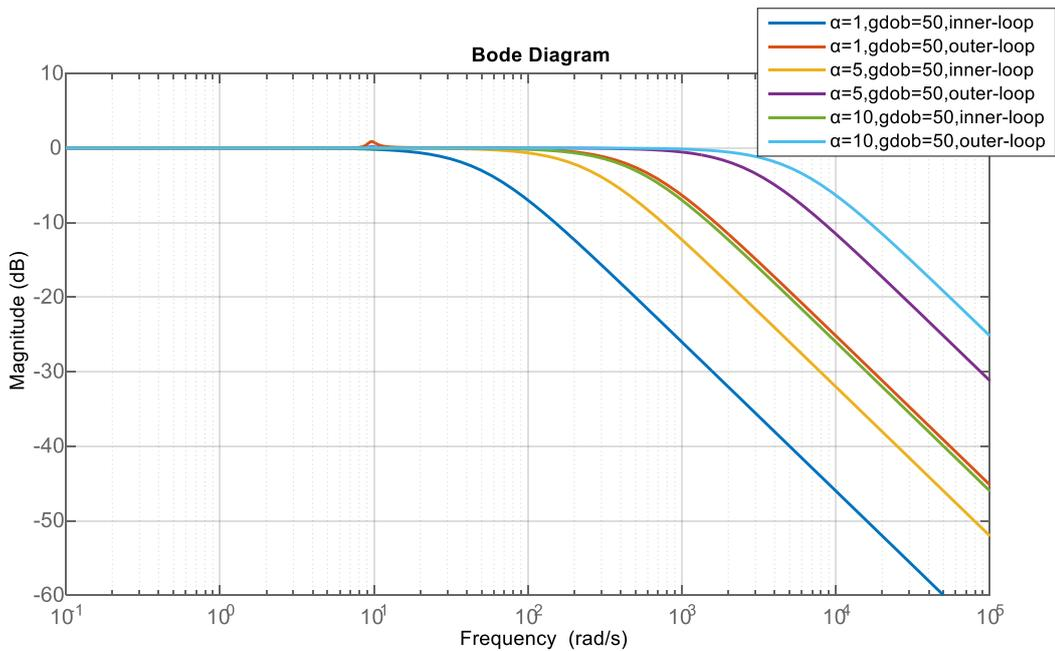
Fig.5.9- Co-sensitivity function frequency response for inner-loop and outer-loop
