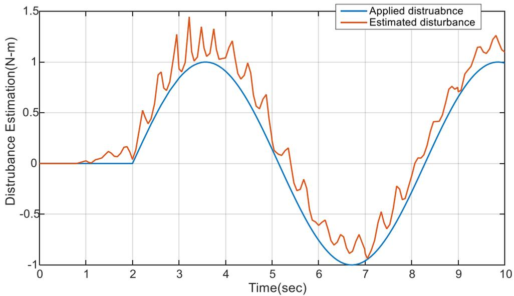
Fig. 4.9- Disturbance estimation plot considering only inner-loop
