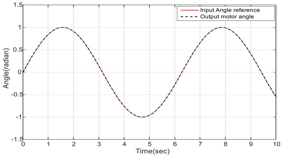
Fig.4.15- Position Control response when sinusoidal input is applied at  $t=0$  and sinusoidal disturbance at  $t=2$  sec
