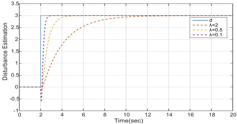
Fig.3.10- Disturbance estimation plots for different  $\lambda$  values
