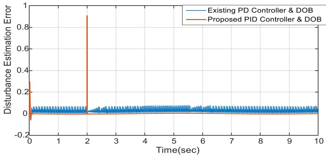
Fig.6.8-Disturbance Estimation Error of the system for sinusoidal input and sinusoidal disturbance applied at t=0 and t=2 respectively
