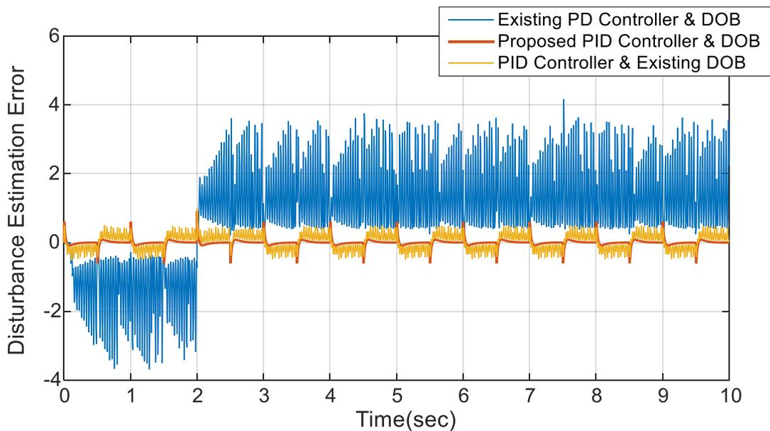
Fig.6.9a-Disturbance Estimation Error of the system for square input and sinusoidal disturbance applied at t=0 and t=2 respectively
