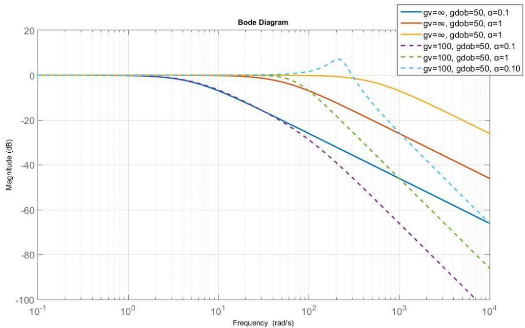
Fig. 5.3- Co-Sensitivity function frequency responses different values of  $\alpha$
