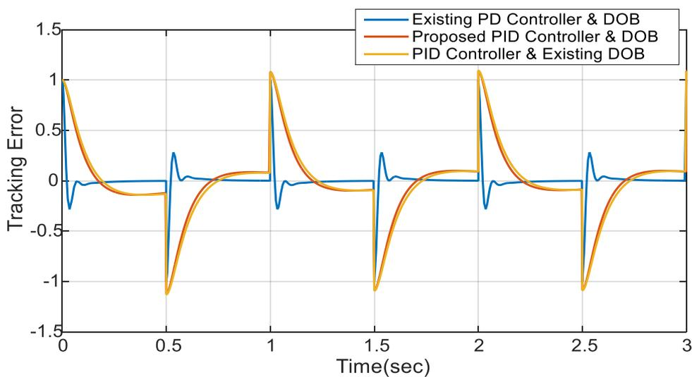
Fig.6.19b- Tracking Error of the system (zoomed up to 3 seconds) for square input and sinusoidal disturbance applied at  $t=0$  and  $t=2$  respectively
