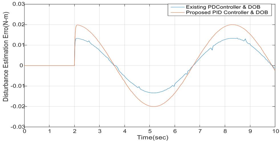
Fig.6.3- Disturbance estimation error when square input as position reference and sinusoidal disturbance is applied at t=0 and t=2 sec respectively
