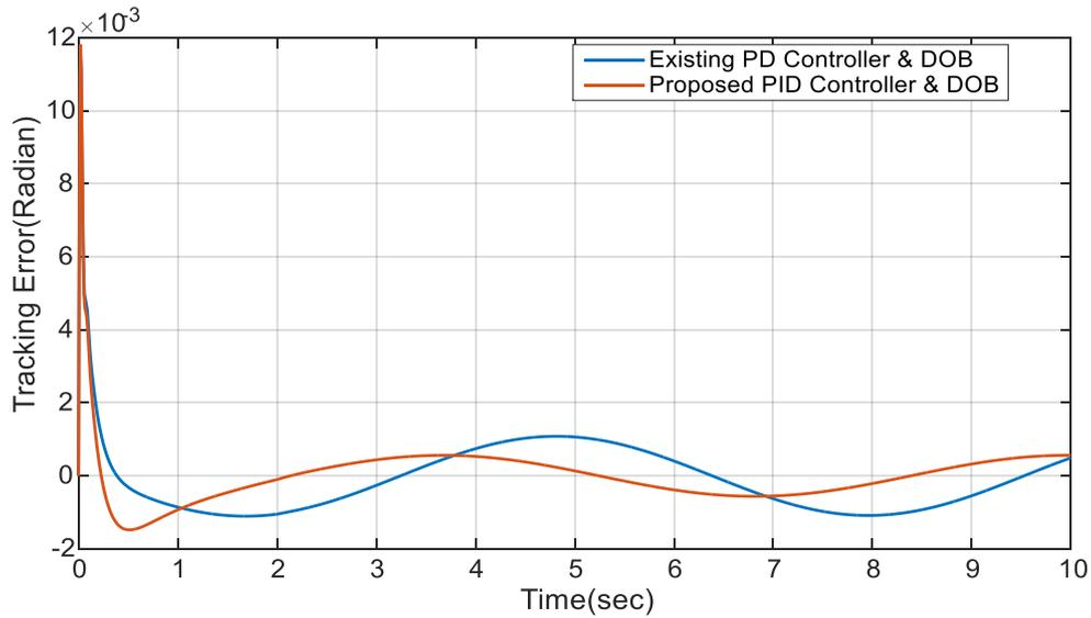
Fig.6.12- Tracking error when sinusoidal input as position reference and sinusoidal disturbance is applied at  $t=0$  and  $t=2$  sec respectively
