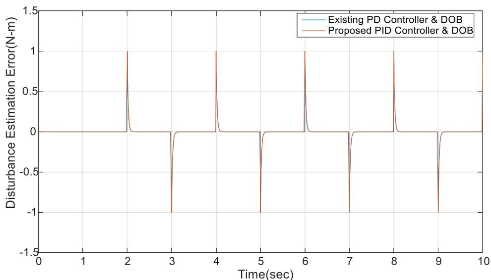
Fig.6.4a- Disturbance estimation error when sinusoidal input as position reference and square disturbance is applied at t=0 and t=2 sec respectively
