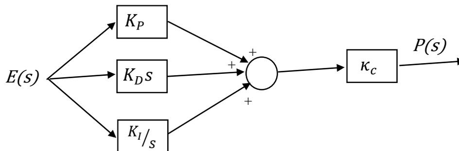
Fig. 5.5- Parallel form PID [27]
