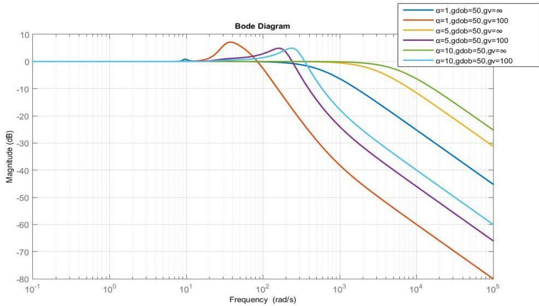
Fig.5.8- Co-sensitivity function frequency response for outer-loop
