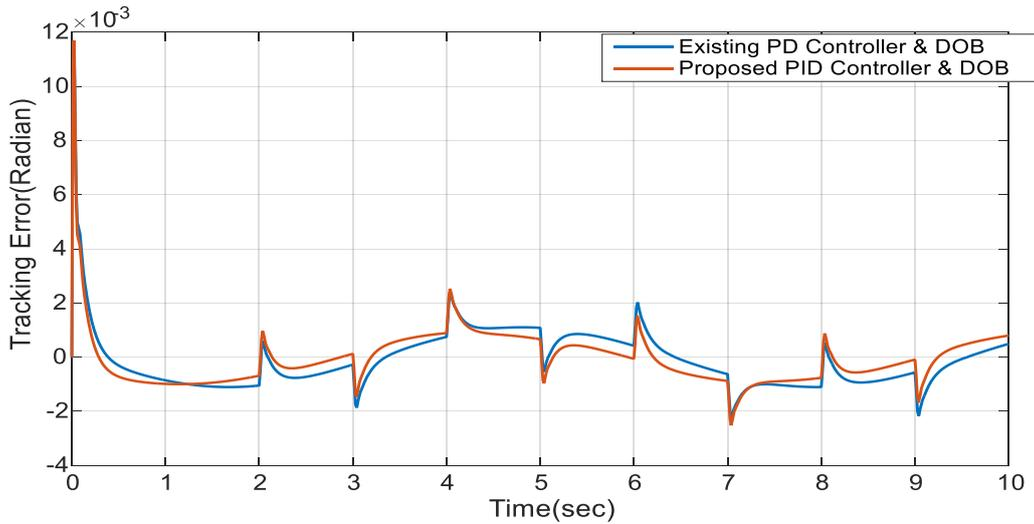
Fig.6.13- Tracking error when sinusoidal input as position reference and square disturbance is applied at  $t=0$  and  $t=2$  sec respectively
