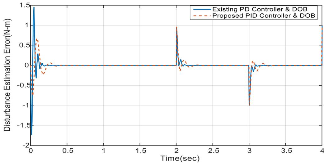
Fig.6.7b- Disturbance Estimation Error of the system for sinusoidal input and square disturbance applied at  $t=0$  and  $t=2$  respectively (zoomed up to 4sec)
