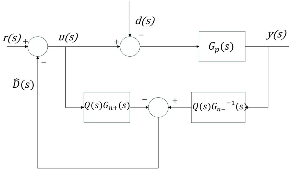
Fig. 3.9- BD of a frequency domain DOB for non-minimum phase linear system [26]
