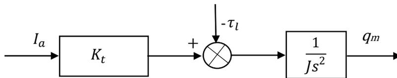
Fig. 4.1- Block diagram of dc servo motor
