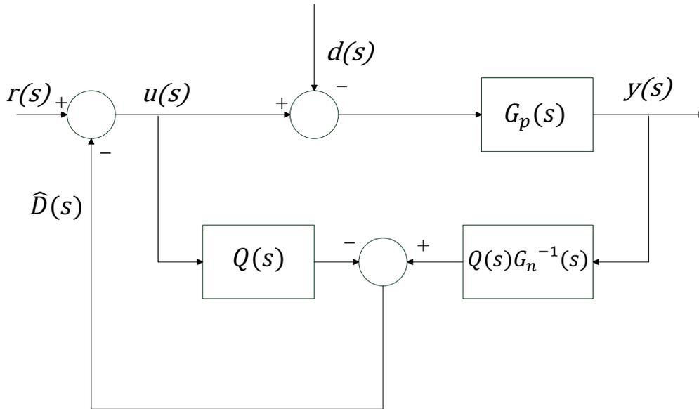
Fig. 3.3a- Block diagram of a frequency domain DOB for minimum phase linear system, an original form [26]
