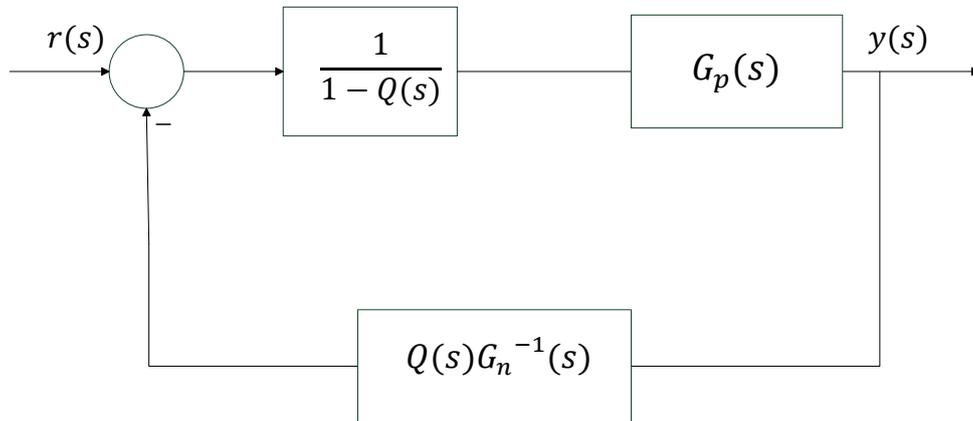
Fig. 3.4- Simplified block diagram of fig. (3.3a)
