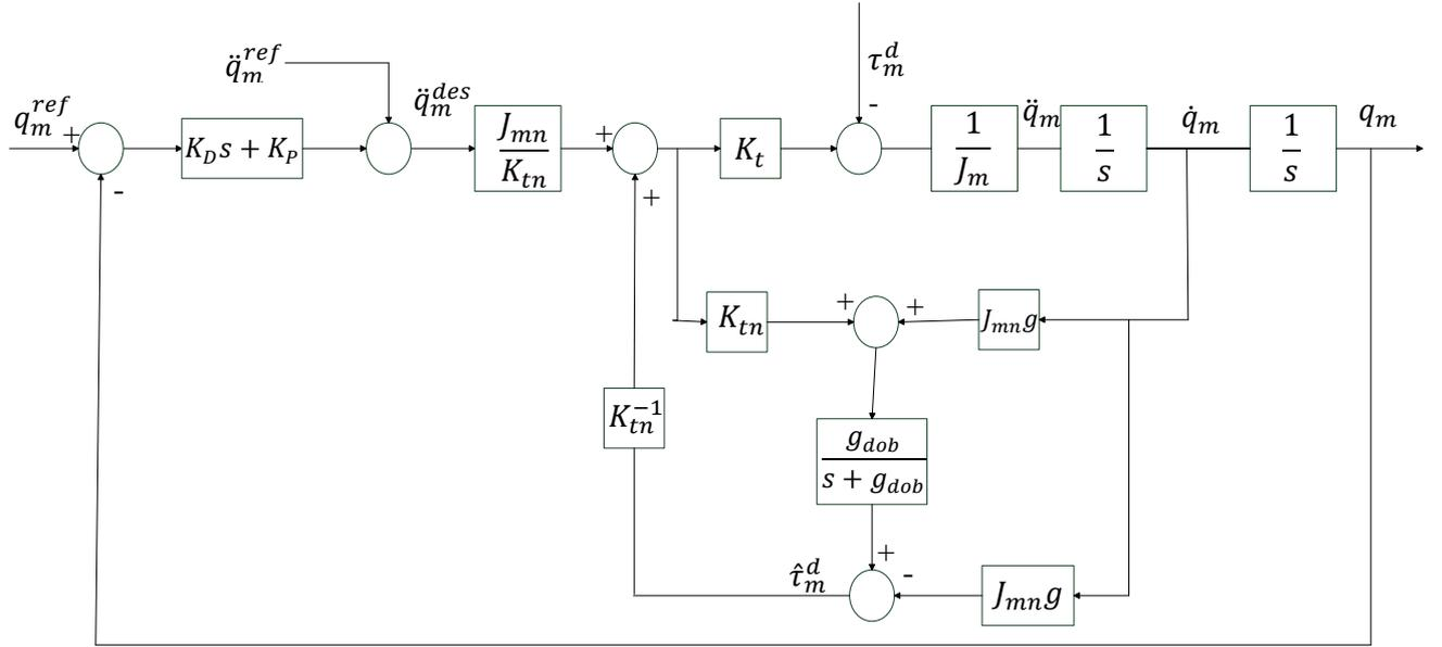
Fig. 4.10- Block diagram of a DOB based robust position control system [24]
