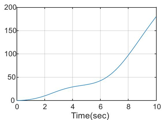
Fig. 4.3- Motor output angle in presence of disturbance
