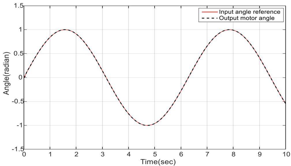
Fig.5.12- Position Control response when sinusoidal input is applied at  $t=0$  and sinusoidal disturbance at  $t=2$  sec
