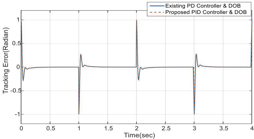
Fig.6.15b- Tracking error when square input as position reference and square disturbance is applied at  $t=0$  and  $t=2$  sec respectively (zoomed up to 4 seconds)
