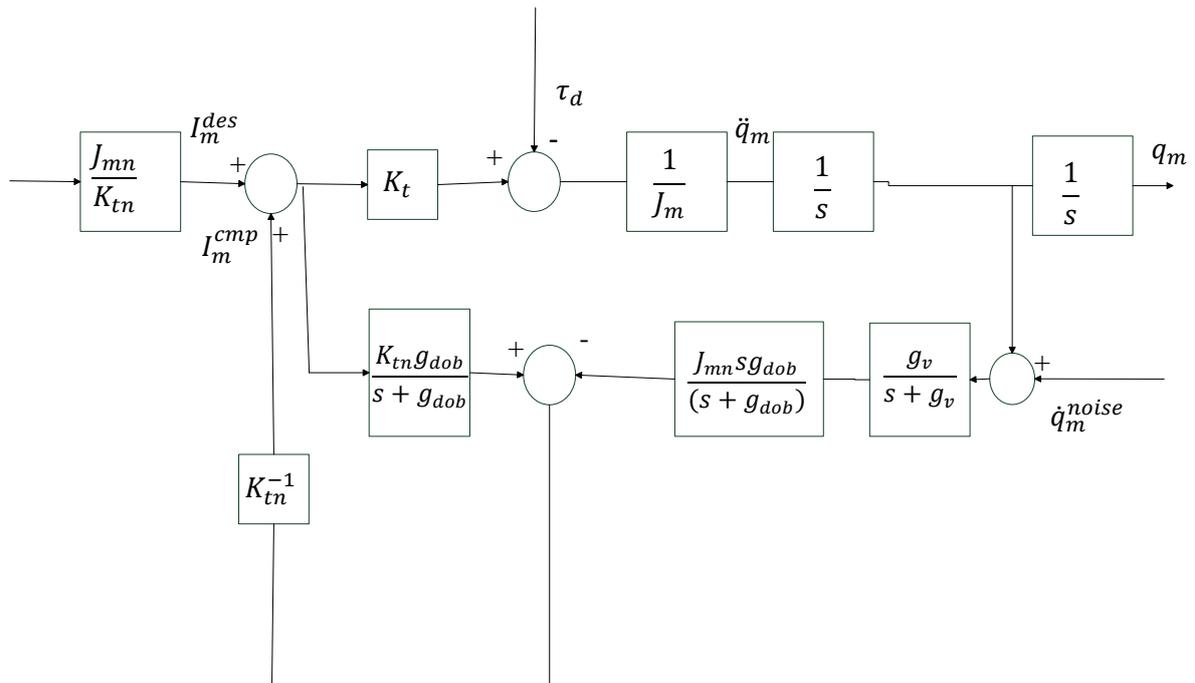
Fig. 5.1- Servo motor system with DOB
