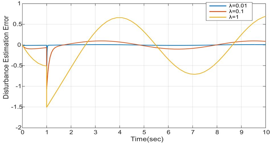
Fig. 3.8- Disturbance estimation error plots for different  $\lambda$  values
