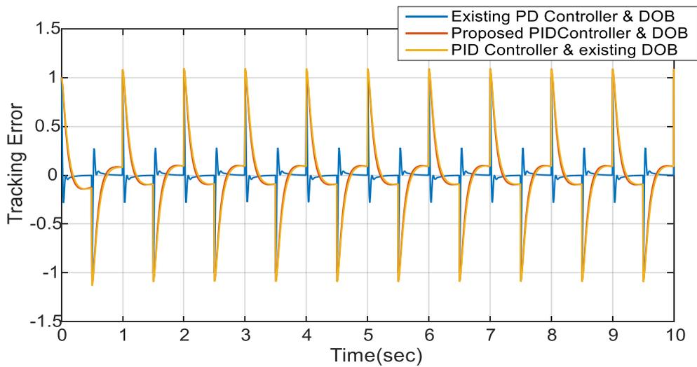
Fig.6.19a- Tracking Error of the system for square input and sinusoidal disturbance applied at  $t=0$  and  $t=2$  respectively
