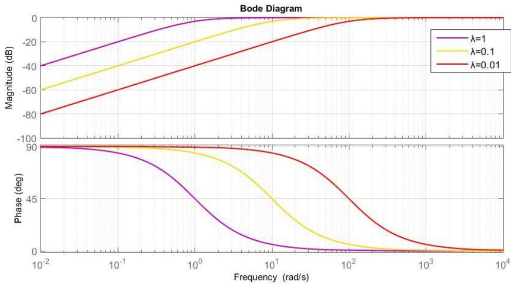
Fig. 3.6- Bode plot for different  $\lambda$  values
