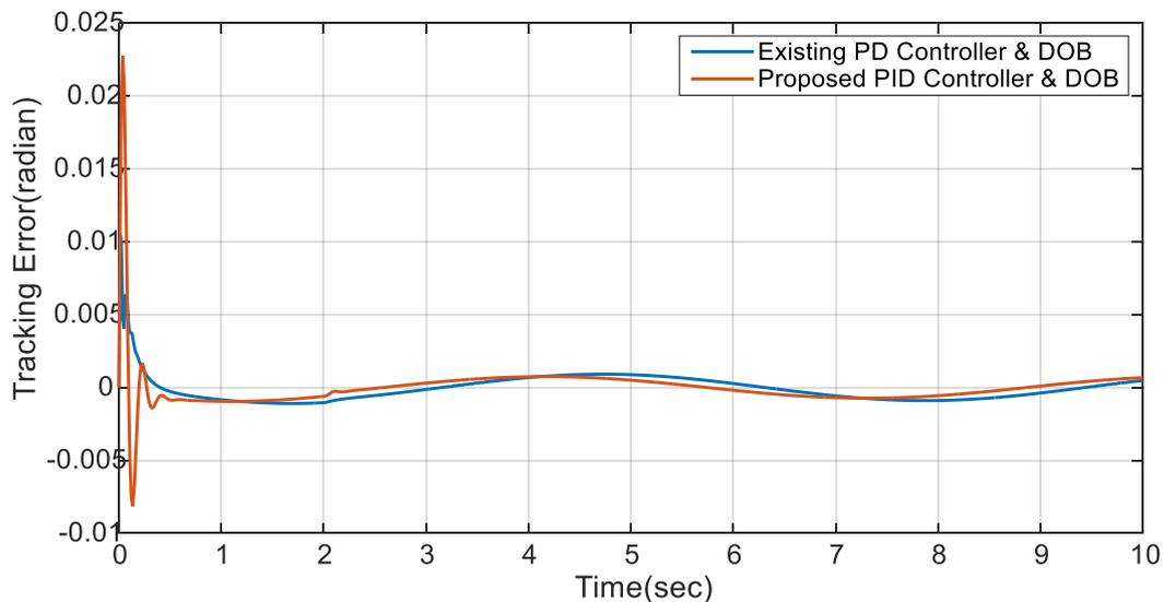
Fig.6.16- Tracking Error of the system for sinusoidal input and sinusoidal disturbance applied at  $t=0$  and  $t=2$  respectively
