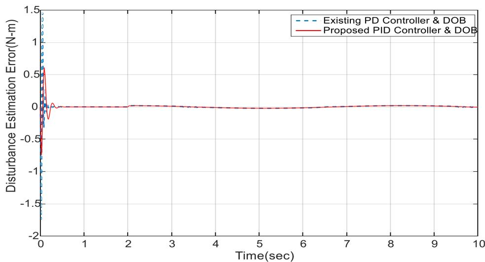
Fig.6.6- Disturbance Estimation Error of the system for sinusoidal input and sinusoidal disturbance applied at t=0 and t=2 respectively
