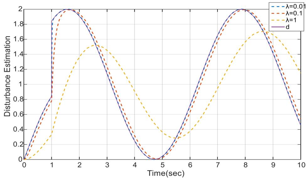
Fig. 3.7- Disturbance estimation plots for different  $\lambda$  values
