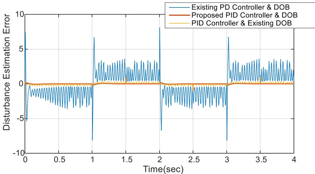
Fig.6.11b- Disturbance Estimation Error of the system for square input and square disturbance applied at  $t=0$  and  $t=1.5$  respectively (zoomed up to 4 seconds)
