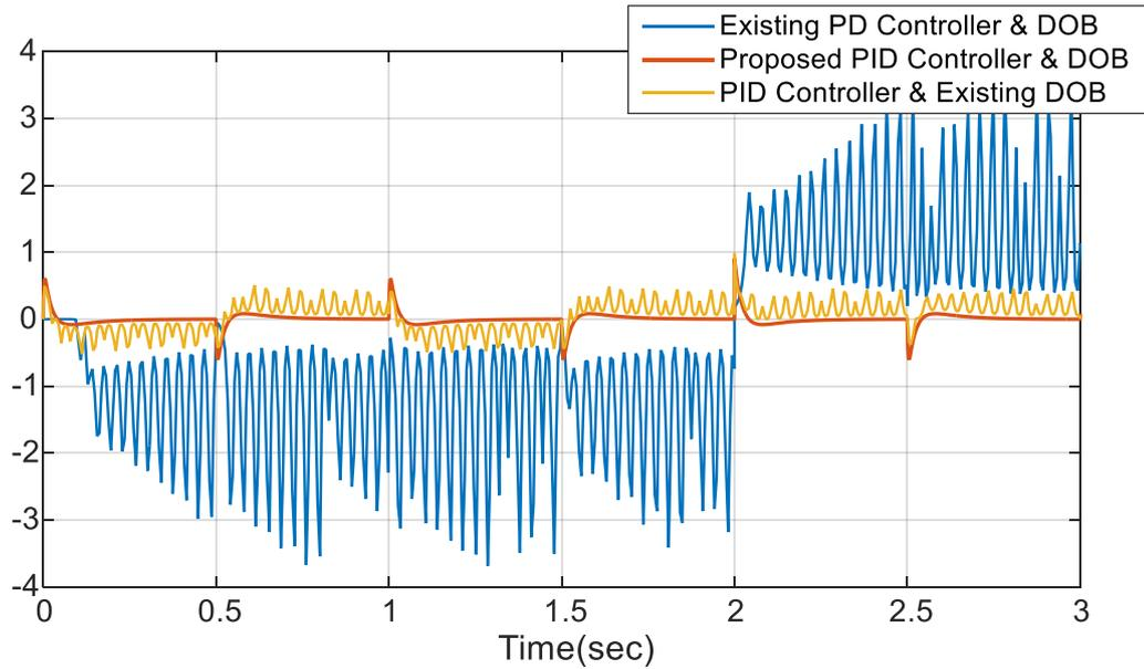
Fig.6.9b-Disturbance Estimation Error of the system for square input and sinusoidal disturbance applied at  $t=0$  and  $t=2$  respectively (zoomed up to 3sec)
