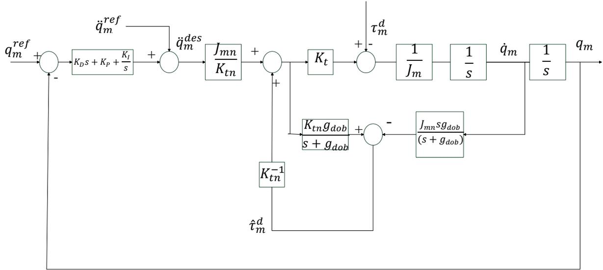
Fig. 5.6- Proposed PID controller & Dob based position control system
