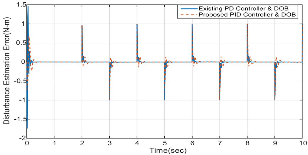
Fig.6.7a- Disturbance Estimation Error of the system for sinusoidal input and square disturbance applied at  $t=0$  and  $t=2$  respectively
