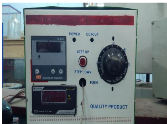
Fig 4.5: PID Temperature Controller
