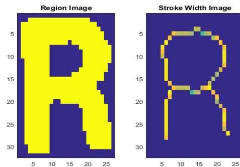
Figure 2: Variation [25] of stroke width image over the region of the left side
