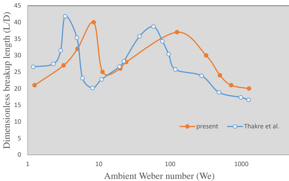
Fig 3.5 Variation of breakup length with respect to Weber number, ( D_j = 5 \text{ mm} )
