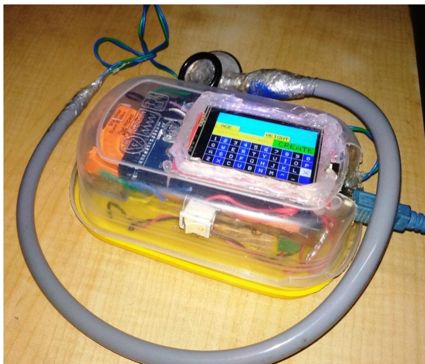
Fig. 5.4 Designed heart sound acquisition system
