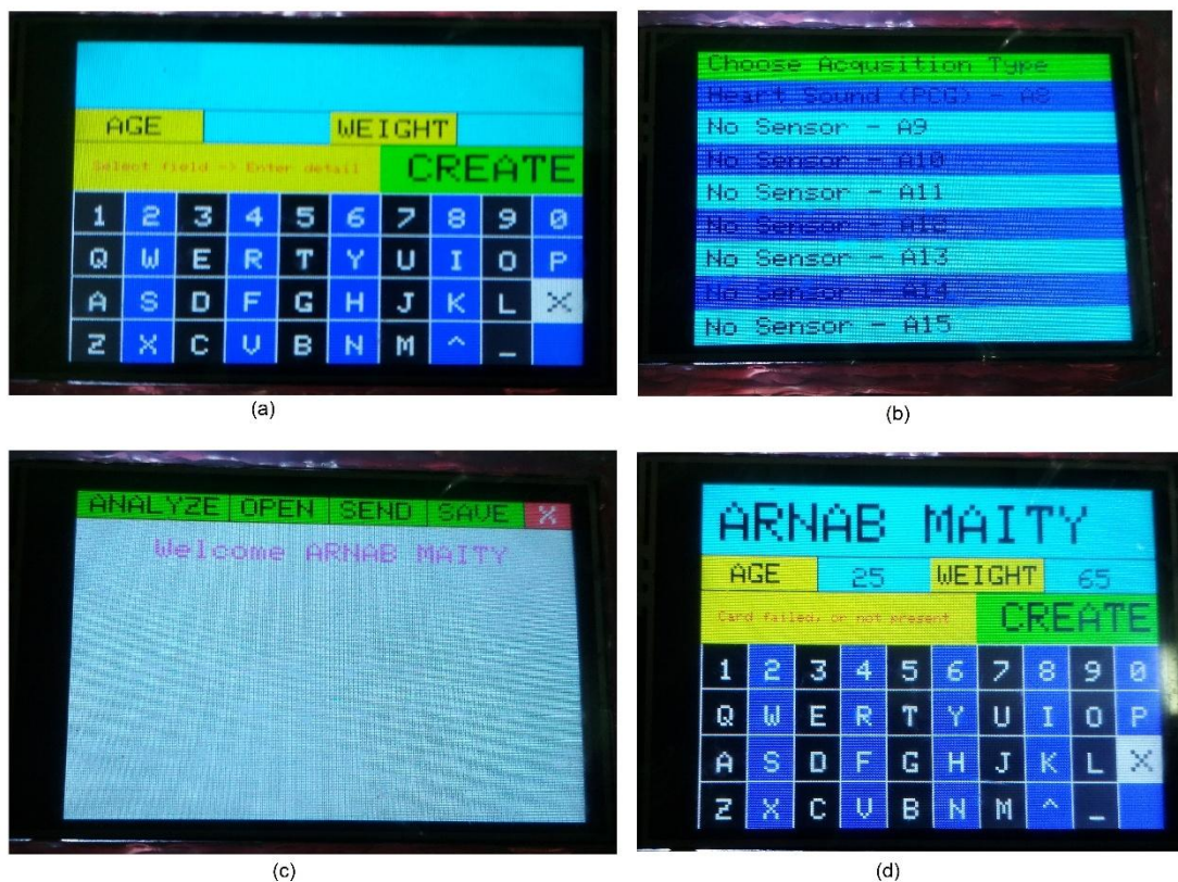
Fig. 5.3 Different Window of the designed UI (a) Patient information window (b) Sensor choice (c) Functional Window (d) Validation error for missing memory card
