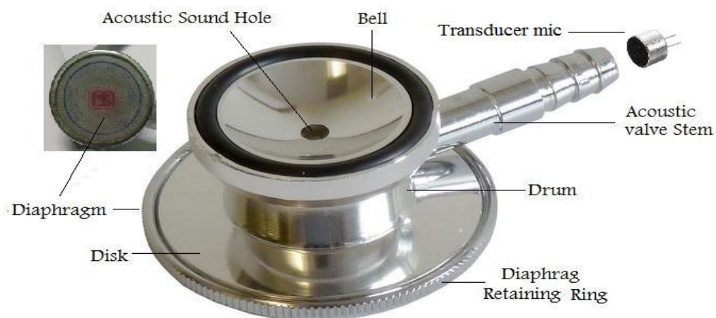
Fig. 4.2 Chest Piece and its different components
