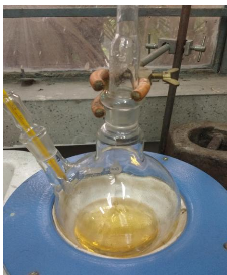
Figure 5.1: Preparation of ester diol
