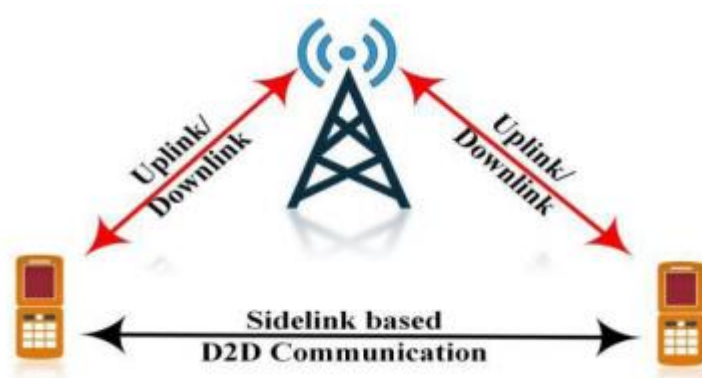
Figure 8: Illustration of Sidelink, Uplink and Downlink in LTE-A network
