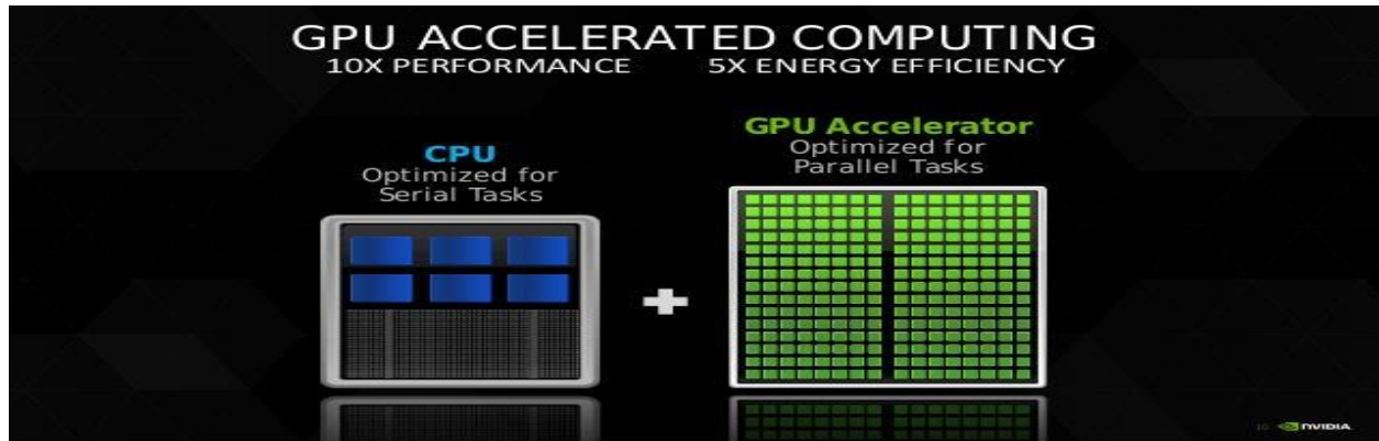
Fig 5.6: Difference between the working of CPU and the GPU
