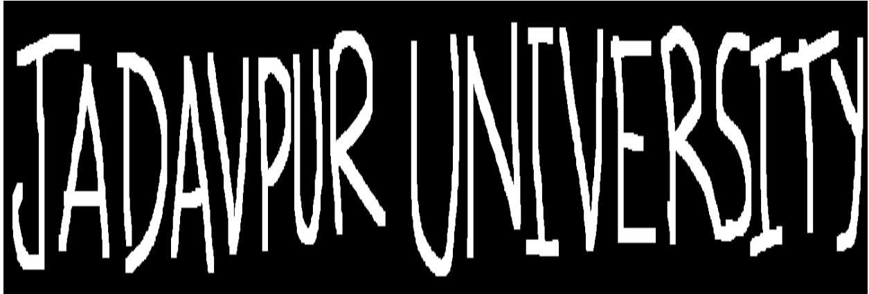
Figure 3.6: After applying dilation on the image
