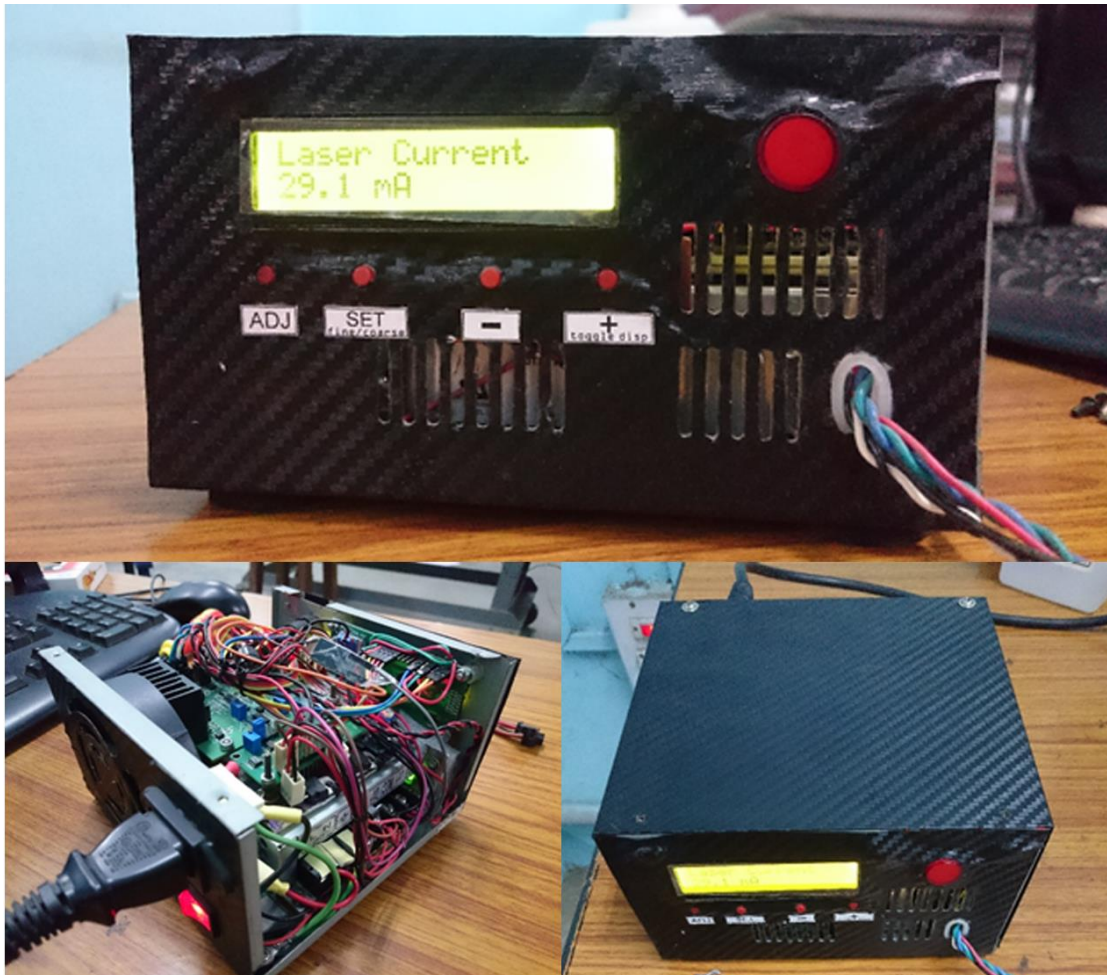
Figure 3.11 - A prototype of the laser power supply
