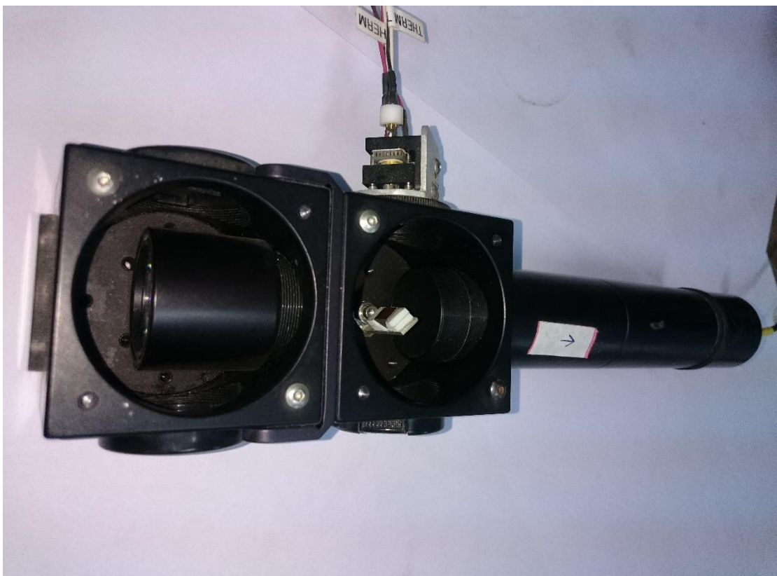
Figure 3.20 - A prototype of the optical head. (In this picture the laser housing is attached)
