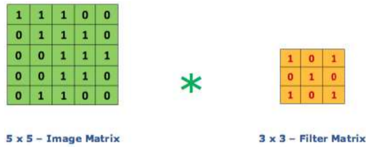
Figure-4.13: Image Matrix Multiplies Kernel or Filter Matrix
