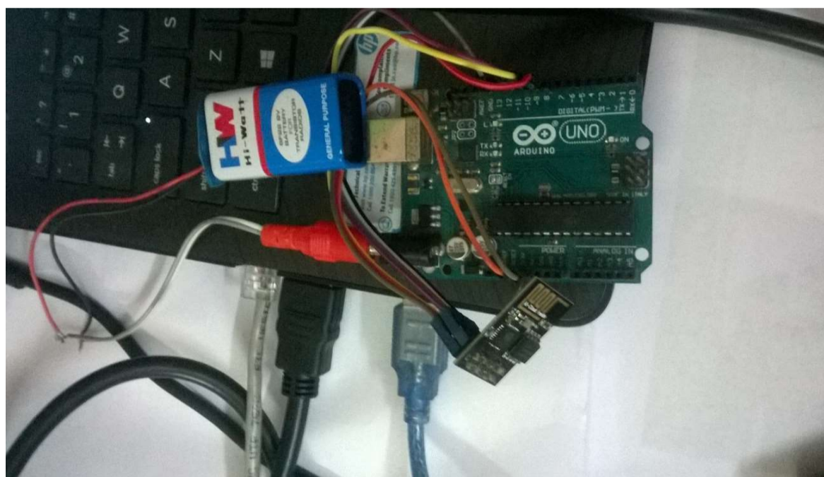
Figure 6.7: Arduino UNO board with Wifi ESP8266 module for wireless communication ESP8266 Module is turned on by using Arduino Uno 3.3V DC Output Pin Figure 6.7 . Arduino board is not delivering sufficient voltage to the ESP8266 module. It was required to use a 3.3 V to power this module. A voltage divider circuit is used to drop the Arduino 5V to ESP8266 3.3 V. After sending AT commands to ESP8266 Module that is connected to Arduino Board and eventually wireless data transfer was successful.
