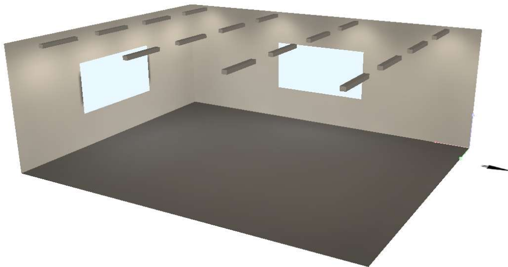
Figure- 7.2 : Daylight Entry through Window (having Certain Dimension) and no Integration of Artificial Light and No Object
