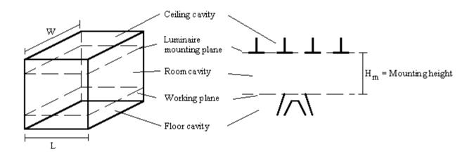
The lumen method is applied only to square or rectangular rooms with a <u>regular</u> <u>array luminaire as shown in Figure below</u>. (lumen)
