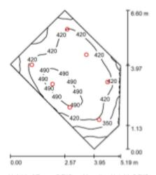
Height of Room: 2.743 m, Mounting Height: 2.743 m, Light loss factor: 0.80
