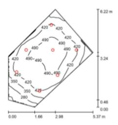
Height of Room: 2.743 m, Mounting Height: 2.743 m, Light loss factor: 0.70
