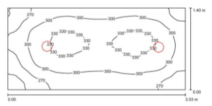
Height of Room: 2.743 m, Mounting Height: 2.743 m, Light loss factor:
