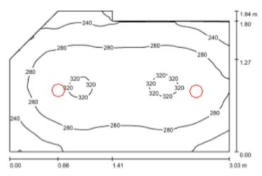
Height of Room: 2.743 m, Mounting Height: 2.743 m, Light loss factor: 0.80
