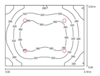
Height of Room: 2.743 m, Mounting Height: 2.743 m, Light loss factor: 0.77
