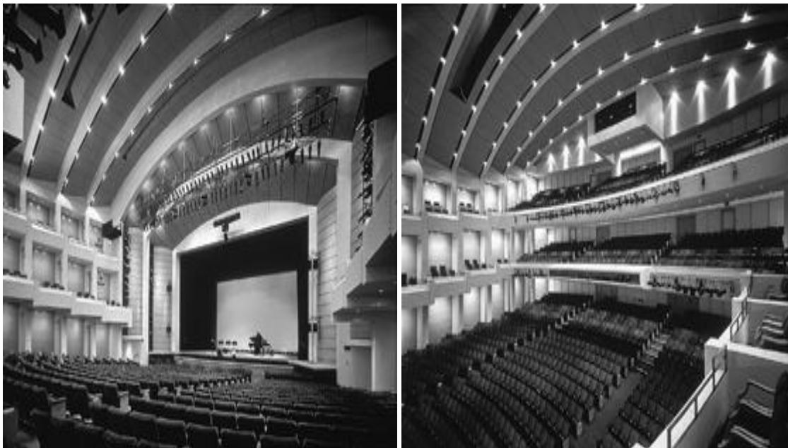
Fig. 4.2: Two views of the Ford Centre for the Performing Arts in Vancouver, British Columbia. The theatre has a traditional proscenium stage, shown here set for a chamber music performance with a large spotlight on the piano. An orchestra pit is located in front of the stage and would be used for musicals, opera, and ballet performances. The interior lighting design features evenly spaced downlights, mounted on the building's structural supports. The lighting provides adequate general illumination and contributes to the pleasantness of the space.
