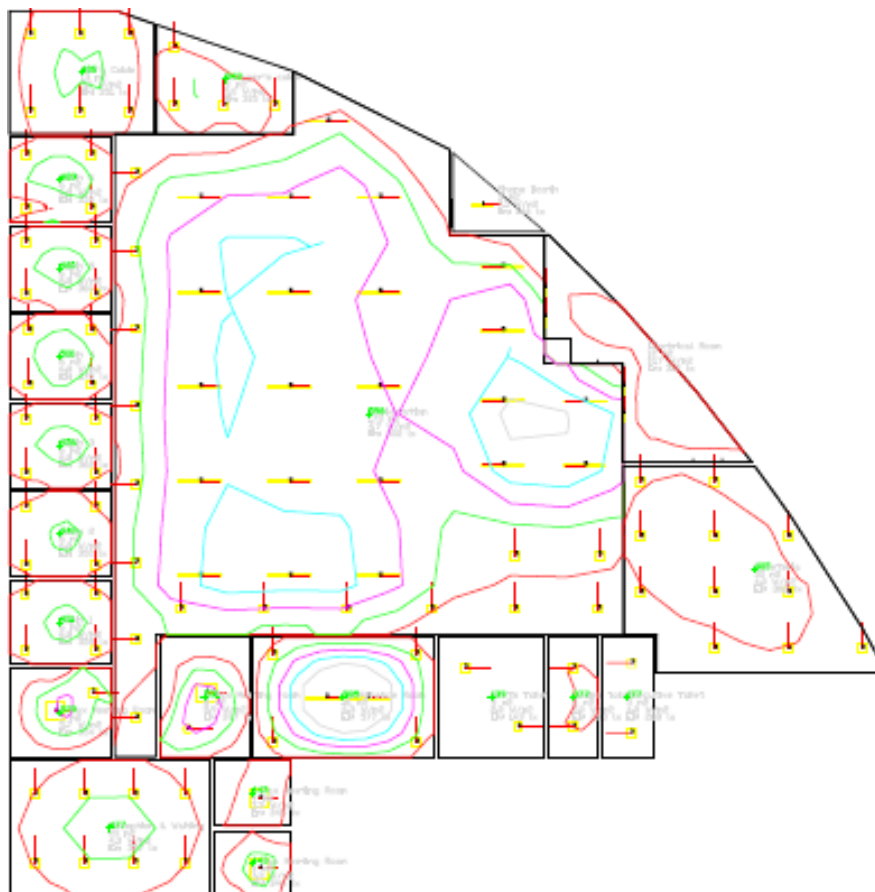
Fig. 7.8 LED Luminaire Layout of Office B Bangalore
