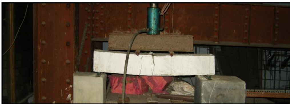
Figure 4.2: Flexural strength test setup for reinforced concrete beam.
