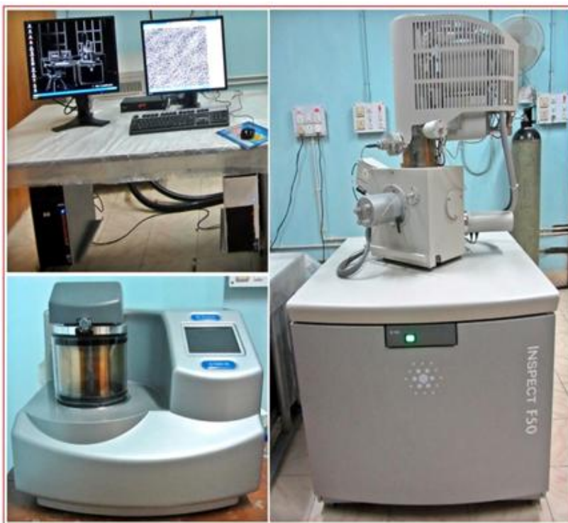
Figure 3.4B: FESEM laboratory test arrangement.
