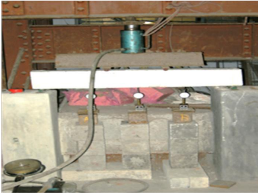
Figure 3.2: Flexural strength test setup for reinforced concrete beam.
