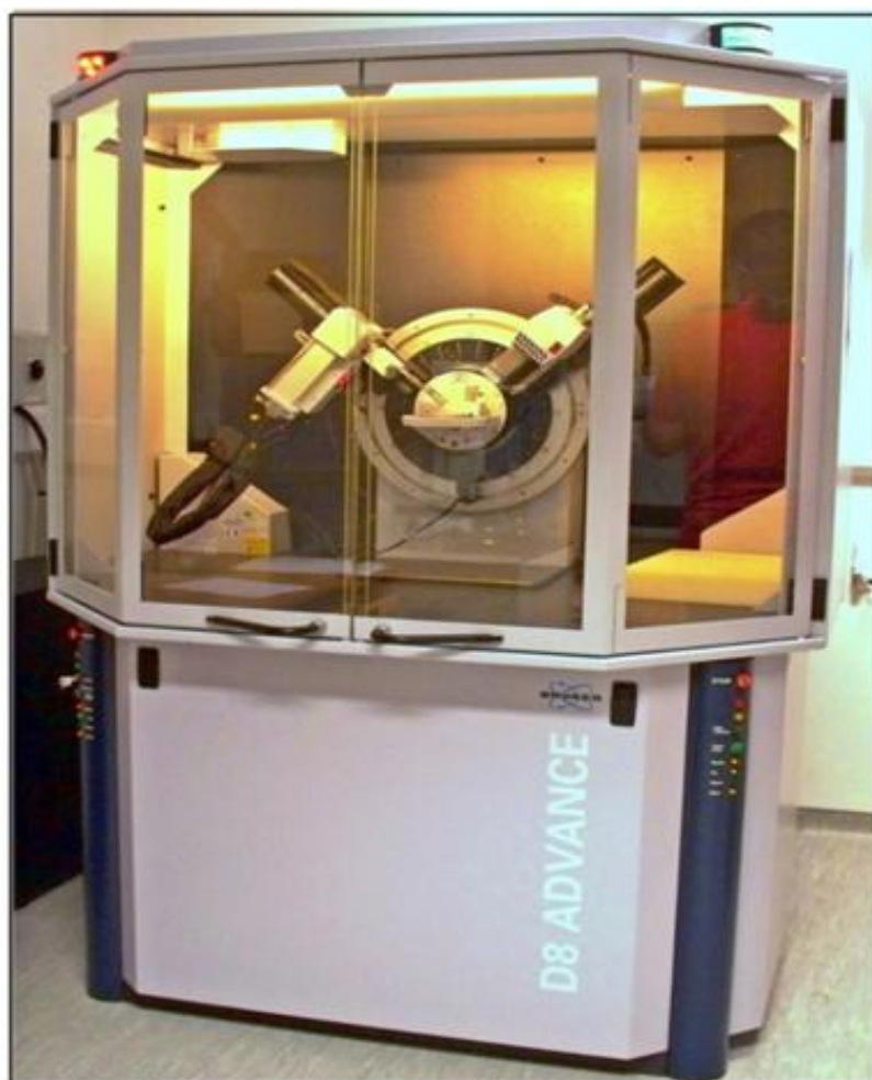
Figure 3.6B: XRD test arrangement.
