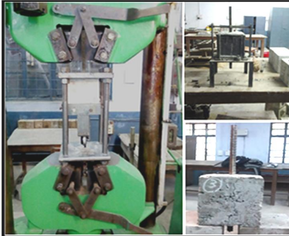
Figure 3.1: Bond strength testing arrangement.
