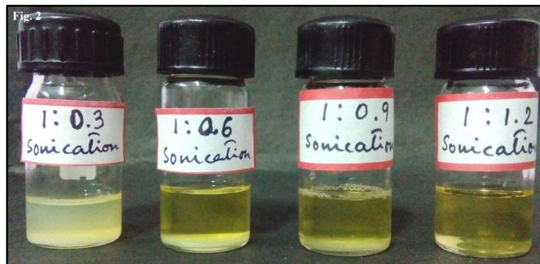
Fig. 4.3.1. Nanoliposomes of black pepper designed with 1% extract using different ratios of soya phosphatidylcholine and Tween 80.
