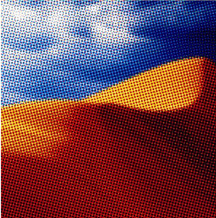
Figure 1.14: A CMYK AM halftone proof with correct screen angles, no Moiré pattern but only Rosette. Screen angles are C 75°, M 105°, Y 90° and K 45°
