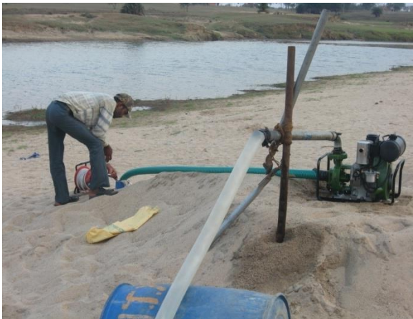
Photo 5.12 : Pumping test photographs in Near Beldihi bridge
