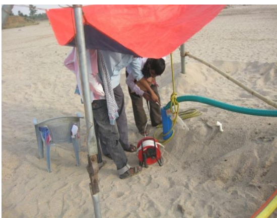
Photo 5.20 : Water table measurement by the help of TLC meter at Teledihi
