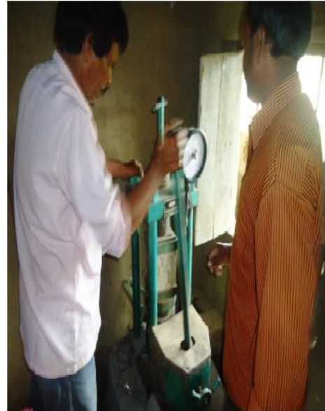
Photo 9.7 : Preparation of concrete test cube and its compressive strength for quality monitoring of the material section of Dam structure
