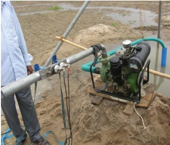
Photo 5.16 : Measuring discharge and sensor setup
