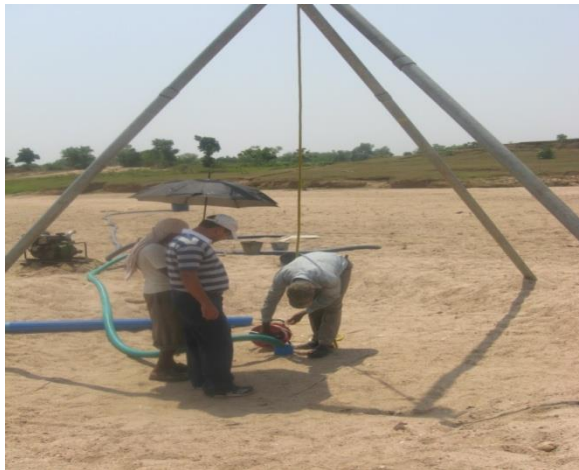
Photo 5.18 : Observation of water table by the help of TLC meter Karadoba
