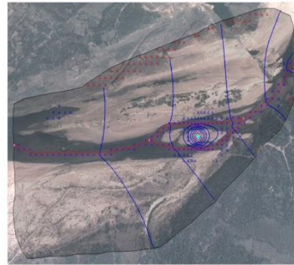
Contour line with color ramp showing head distribution for layer 2 for PT-4
