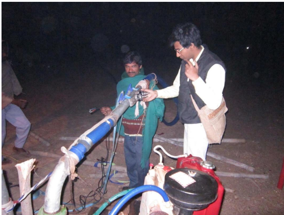
Photo 8.1: Withdrawal rate measurement at 2 nd pumping test in Damodar river
