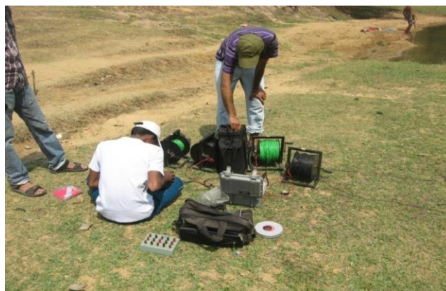
Photo 5.2: Geophysical Data collection using (VES) Instrument
