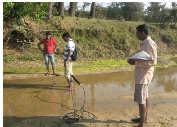
Photo 5.24 : Measurement of Velocity in between Beldihi bridge and Baligara
